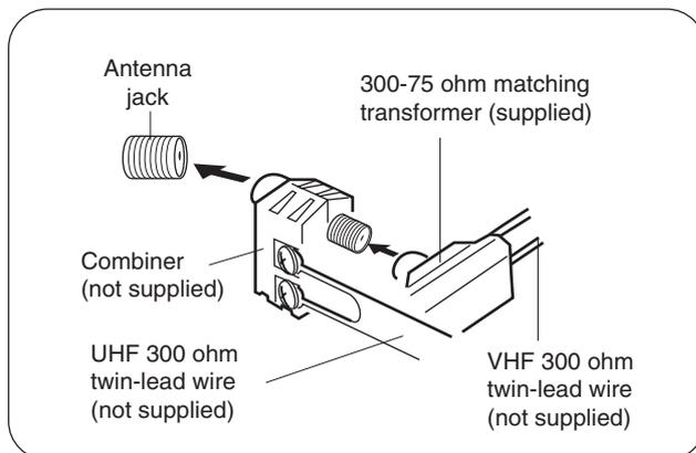
Connect the UHF 300 ohm twin-lead wire to the combiner (not supplied). Connect the VHF 300 ohm twin-lead wire to the 300-75 ohm matching transformer. Attach the transformer to the combiner, then attach the combiner to the antenna jack.
