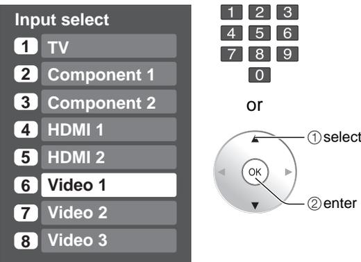
Press corresponding NUMBER button on the remote control to select the input of your choice.
