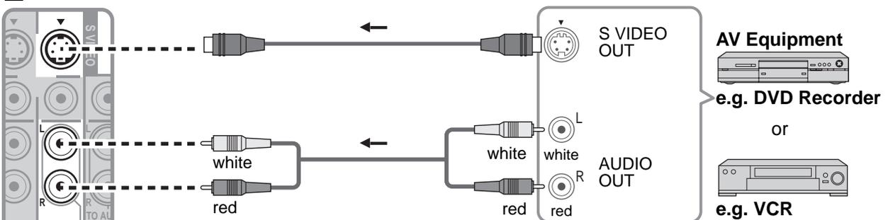
● The S Video input will override the composite video signal when S Video cable is connected. Connect either S Video or Video cable.
