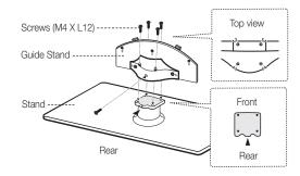
1. Connect the Guide Stand to the Stand using five screws (M4 X L12) as shown.
