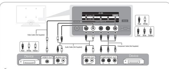
COMPONENT IN / AV IN: When connecting to AV IN, the color of the AV IN [Y/VIDEO] jack (green) will not match the video cable (yellow).
