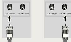
➤ If both ANT1 IN(AIR) and ANT2 IN(CABLE) are connected, select the antenna input you want. If the antenna input is not selected properly, noise may appear on the screen.
