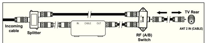
After you have made this connection, set the A/B switch to the “A” position for normal viewing. Set the A/B switch to the “B” position to view scrambled channels. (When you set the A/B switch to “B”, you will need to tune your TV to the cable box’s output channel, which is usually channel 3 or 4.)
