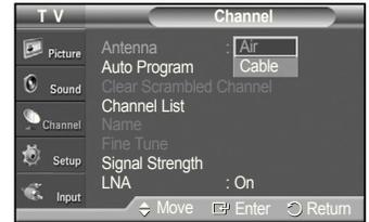
➤ If the antenna is connected to ANT1 IN(AIR), select **Air** and if it is connected to ANT2 IN(CABLE), select **Cable**.
