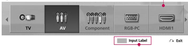
Disconnected inputs are inactive (grayed out)
