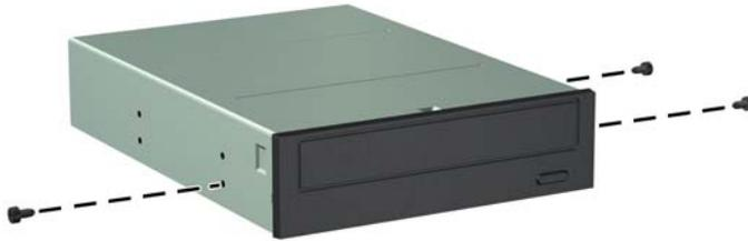
5. Position the mounting screws on the drive into the J-slots in the drive bay. Then slide the drive toward the front of the computer until it stops.
