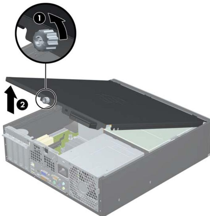
To install the access panel, reverse the removal procedure.
