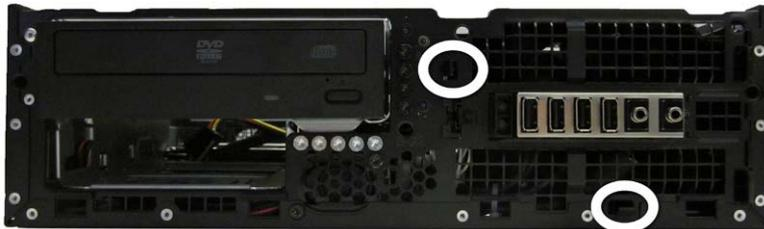
7. Pull the assembly toward the rear of the unit, and then lift it out of the chassis.
