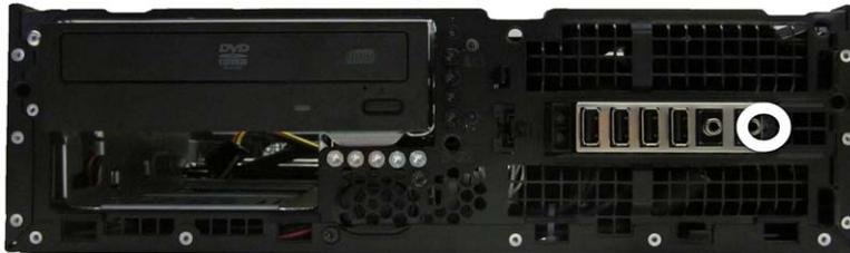
8. Route the cables through the slots beneath the drive cage, pull the assembly (right side first) into the chassis, and then remove the assembly from the computer.
