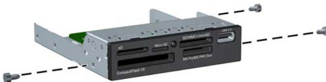
4. Position the mounting screws on the drive into the J-slots in the drive bay. Then slide the drive toward the front of the computer until it stops.
