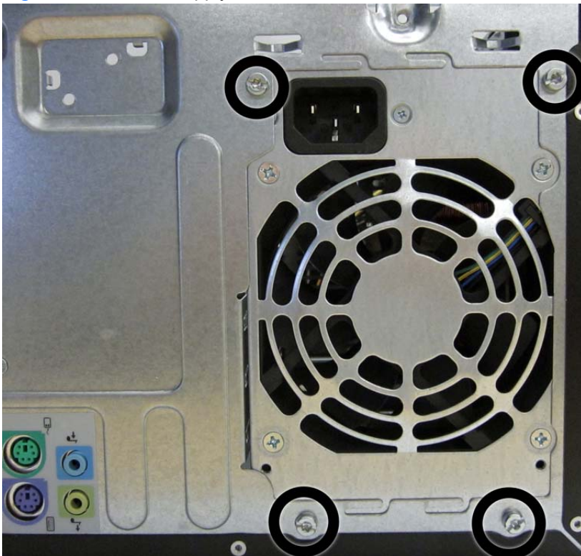
Figure 7-34 Power supply screws
