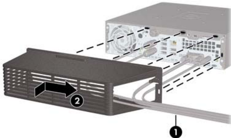
Figure 9-45 Installing a Port Cover
