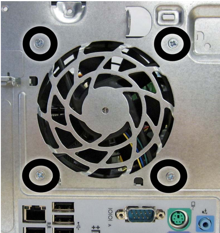
Figure 7-32 Rear fan screws
