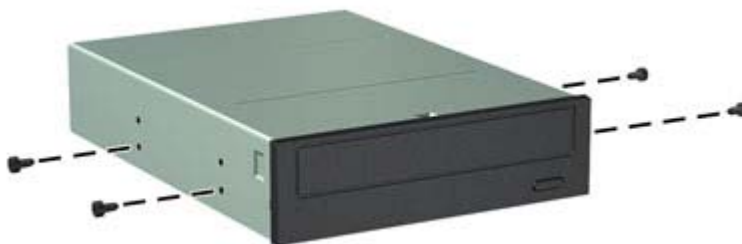
Figure 8-17 Installing Guide Screws in the Optical Drive
