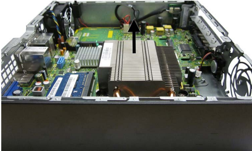
Figure 9-26 Removing the heat sink
