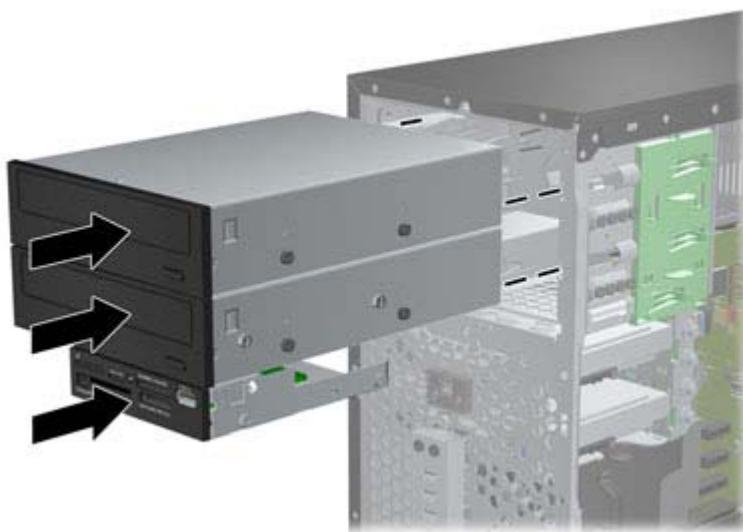
Figure 7-19 Sliding the Drives into the Drive Cage
