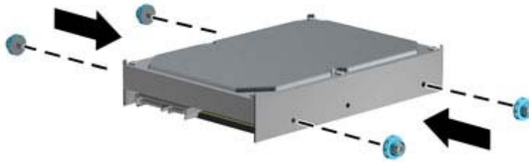
Figure 7-22 Installing Isolation Mounting Guide Screws in a 3.5-inch Drive
