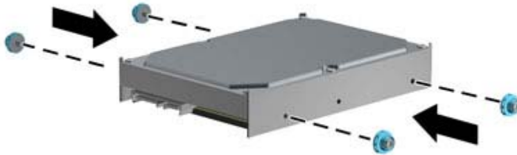
Figure 8-26 Installing Hard Drive Guide Screws
