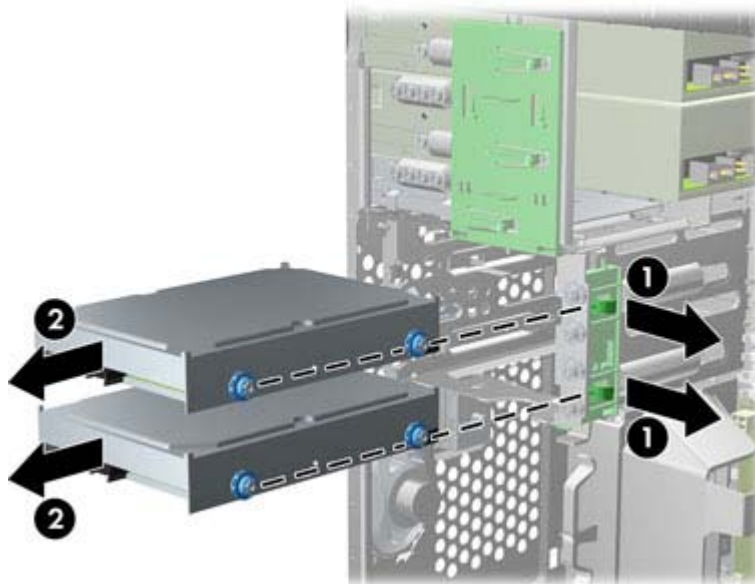
Figure 7-21 Removing a Hard Drive
