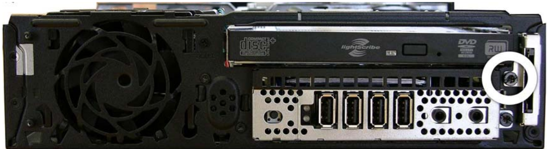
Figure 9-22 Removing the card reader screw
