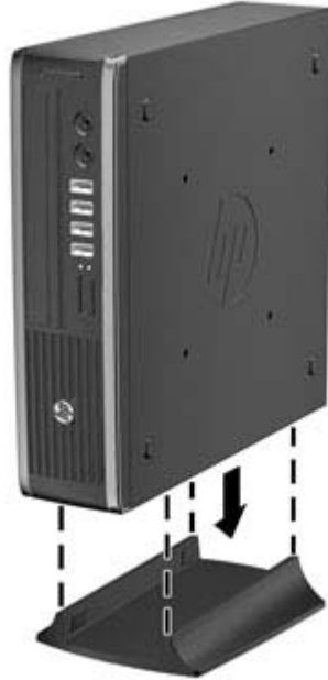
Figure 9-44 Placing the computer on the stand
