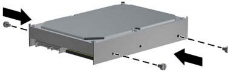
Figure 6-26 Installing Standard Guide Screws
