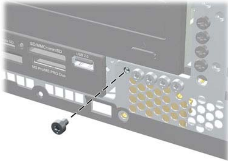
Figure 8-3 Retrieving the Front Bezel Security Screw
