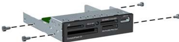
Figure 8-21 Installing Guide Screws (Media Card Reader Shown)
