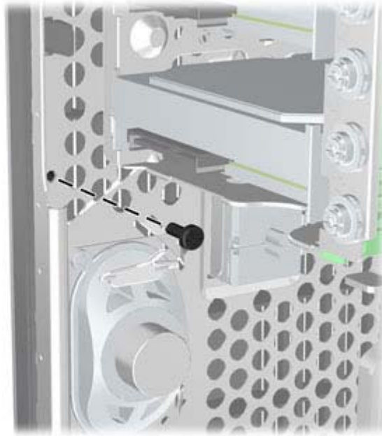
Figure 7-4 Installing the Front Bezel Security Screw
