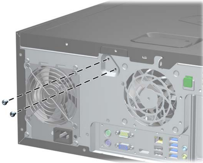
Figure C-2 Removing the Smart Cover Lock Screws from the Microtower
