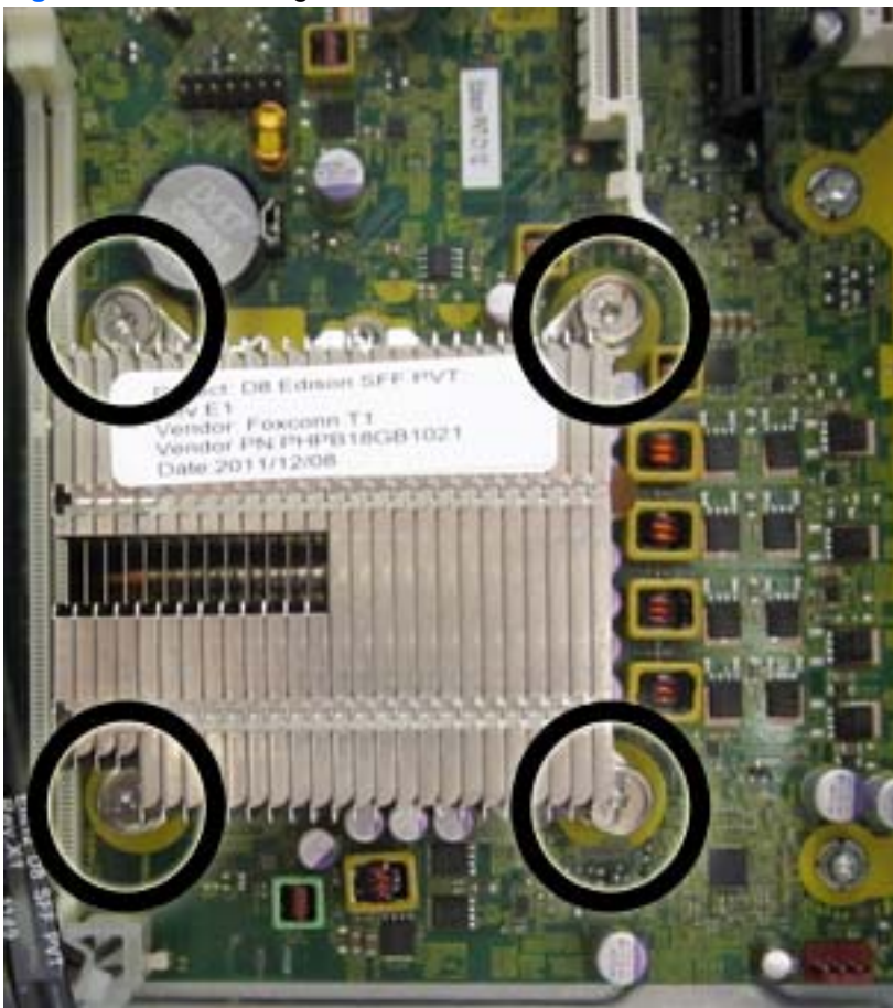
Figure 7-30 Removing the heat sink
