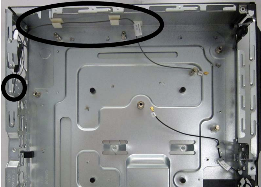
Figure 9-41 Removing the rear antenna – inside
