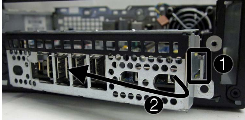
Figure 9-35 Removing the I/O panel
