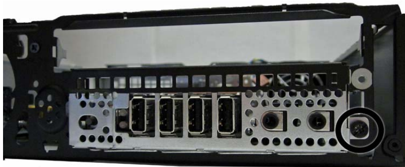
Figure 9-34 I/O panel screw
