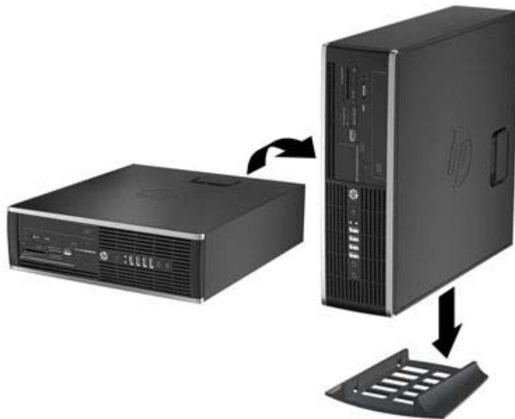
Figure 8-40 Changing from Desktop to Tower Orientation
