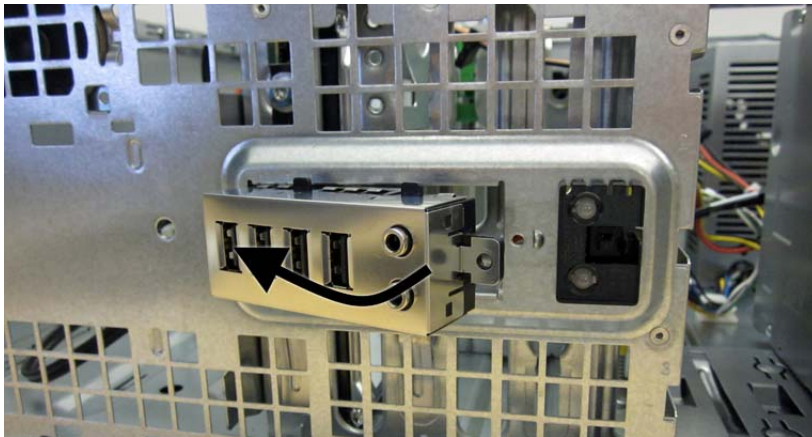
Figure 6-30 Removing the front I/O, USB, power switch assembly
