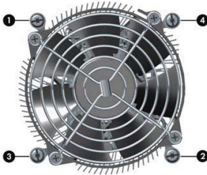
Figure 6-34 Loosening the fan sink screws
