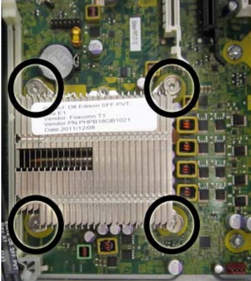
Figure 8-35 Removing the heat sink
