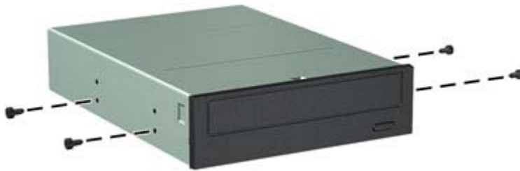
Figure 7-18 Installing Guide Screws (Optical Drive Shown)
