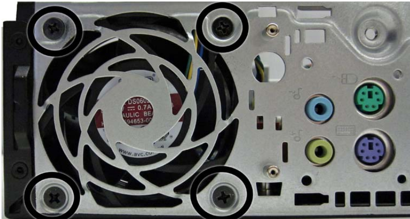
Figure 9-37 Removing the rear fan screws
