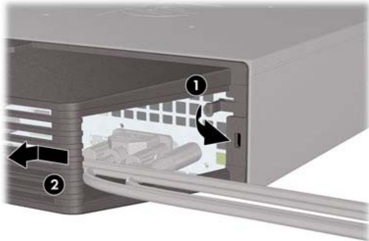
Figure 9-46 Removing a Port Cover
