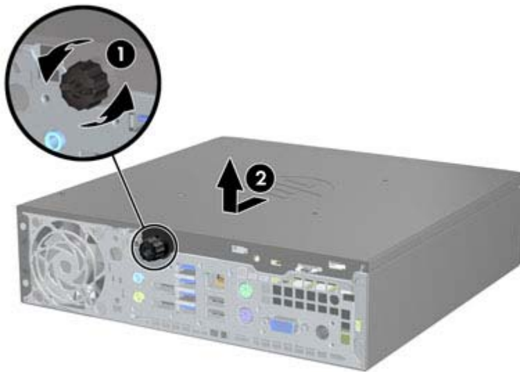
Figure 9-1 Removing the Computer Access Panel
