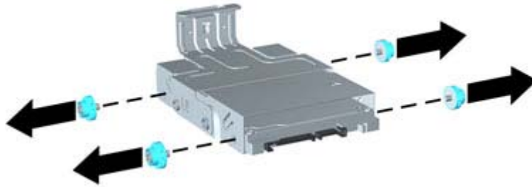
Figure 9-16 Removing the guide screws
