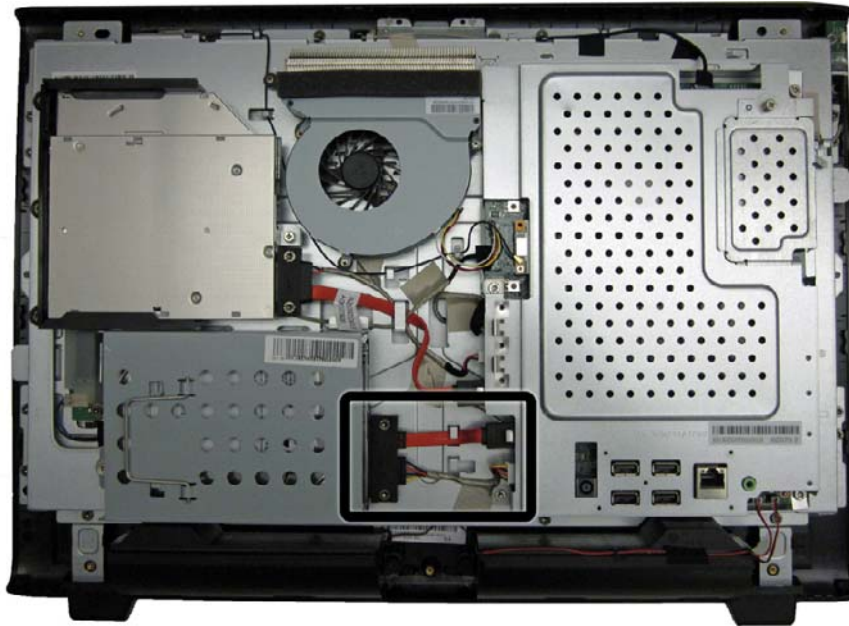
Figure 6-36 Hard drive cable location
