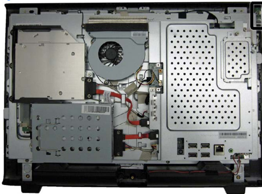
Figure 6-44 Power button board location
