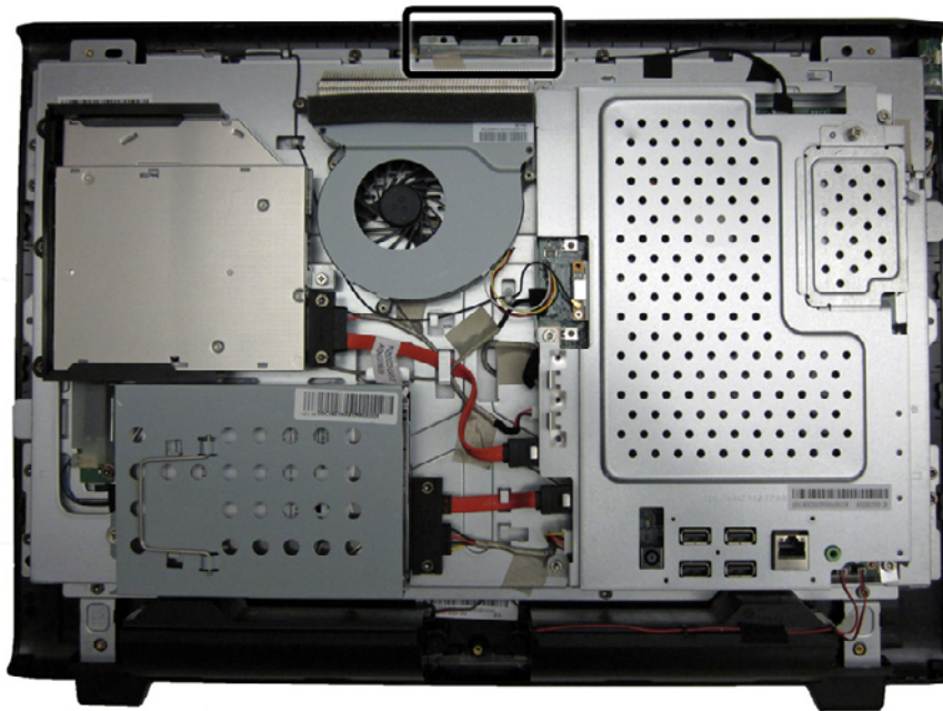
Figure 6-32 Webcam module location
