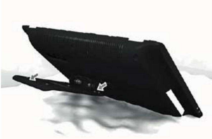
Figure 6-7 Removing the stand
