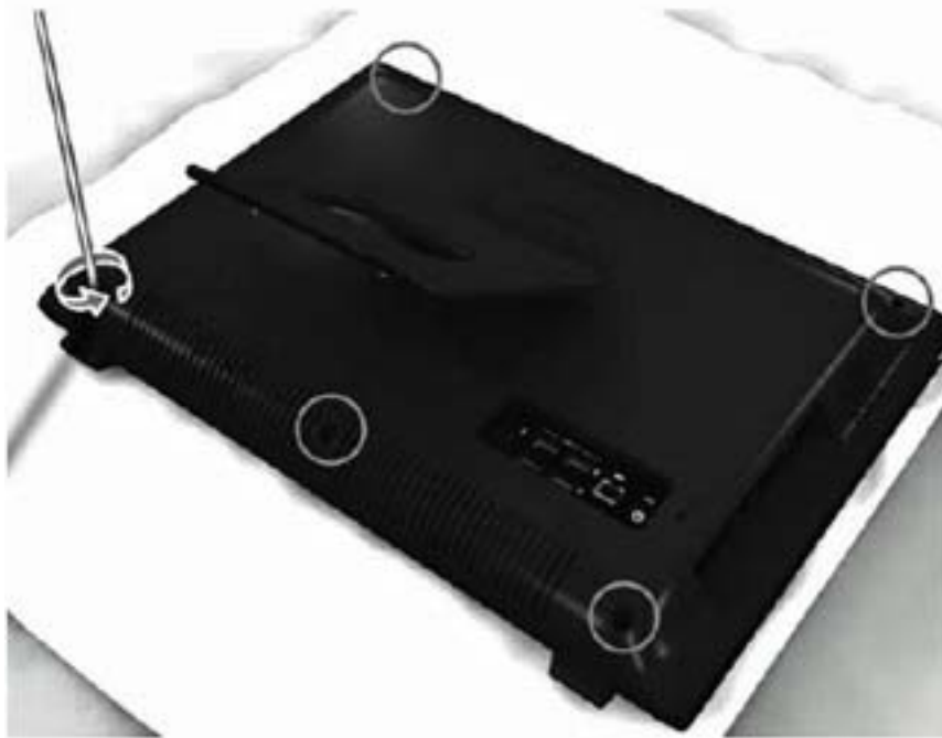
Figure 6-2 Removing the rear cover screws
