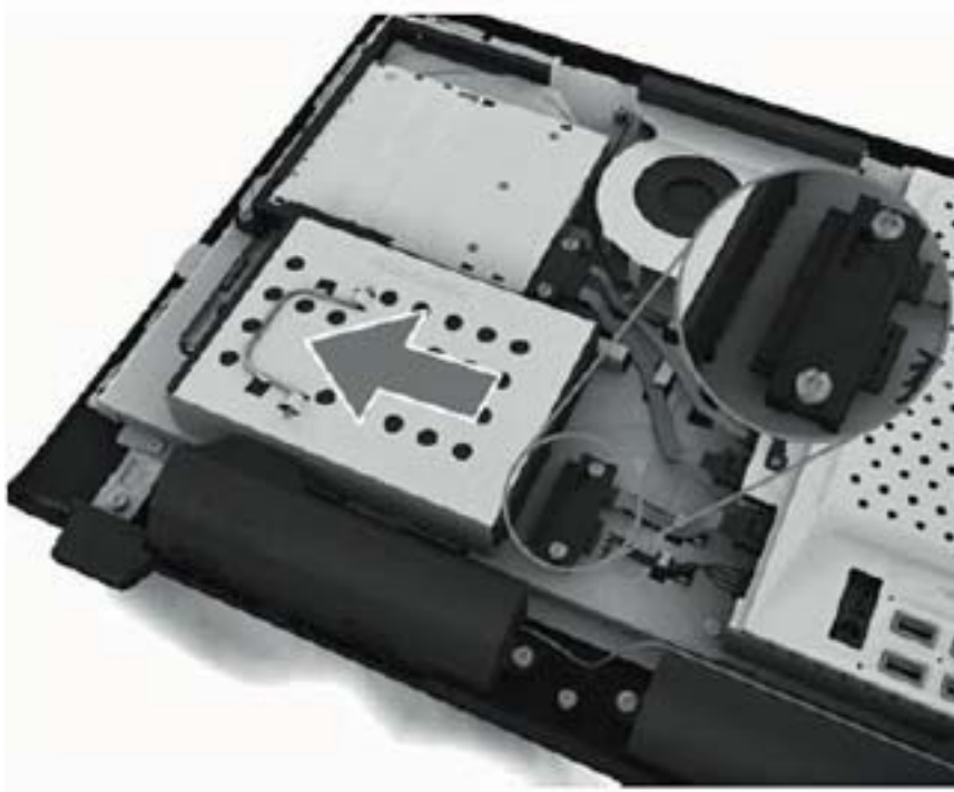
Figure 6-13 Sliding the hard drive to disconnect the cables
