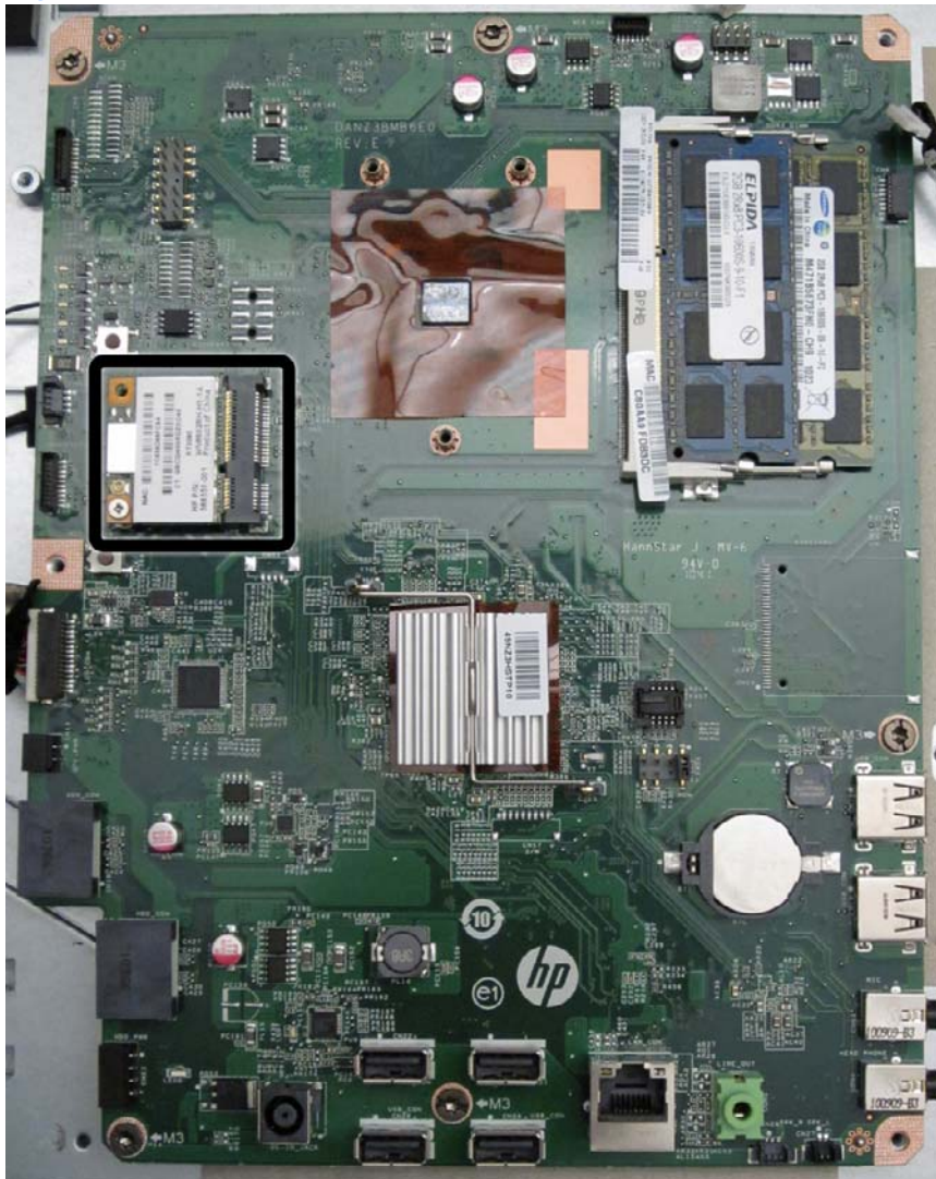
Figure 6-50 WLAN module location
