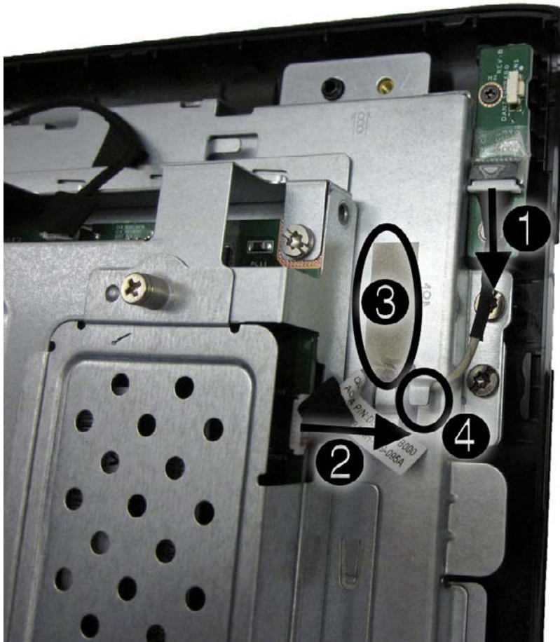
Figure 6-46 Removing the power button board cable
