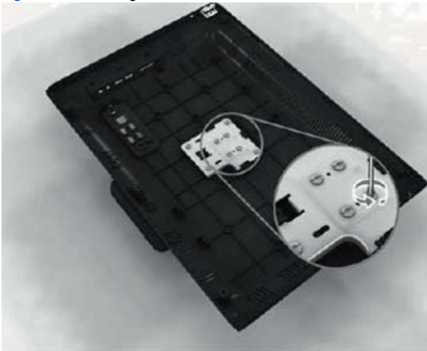
Figure 6-6 Removing the stand screws
