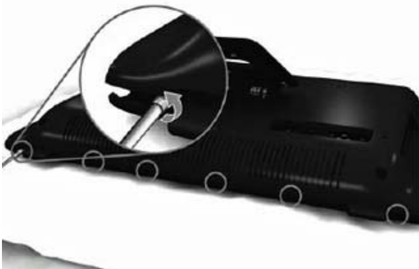
Figure 6-3 Prying the rear cover loose
