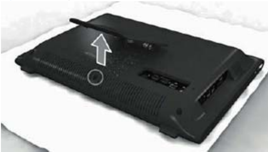
Figure 6-1 Lifting the stand
