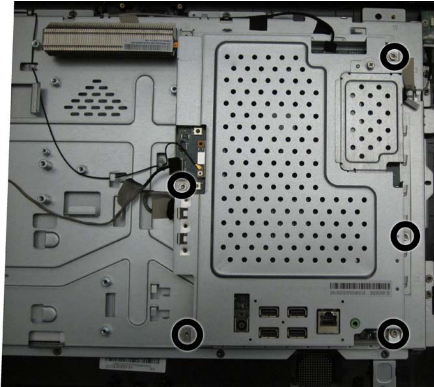
Figure 6-48 Removing the system board shield
