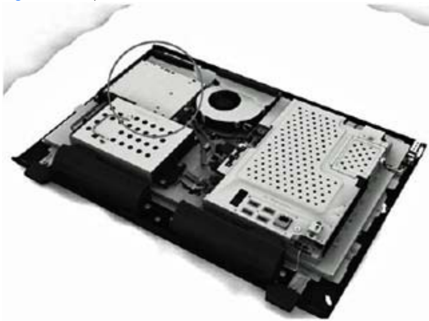
Figure 6-8 Optical drive location
