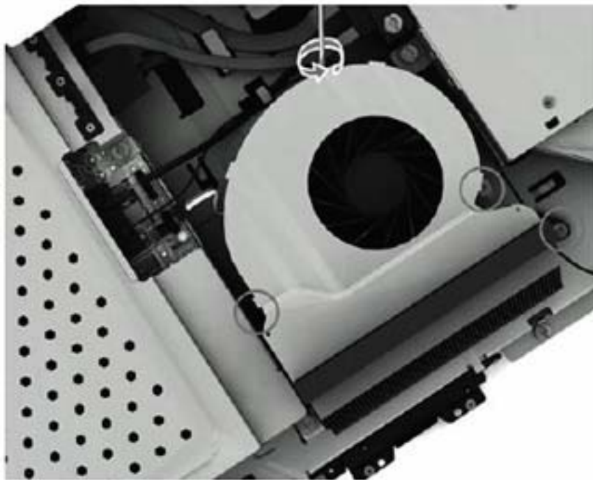
Figure 6-24 Removing the fan screws
