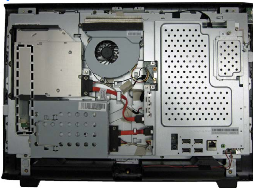
Figure 6-41 Inverter board location
