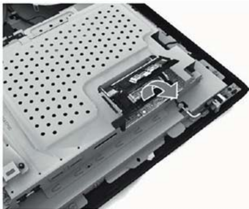
Figure 6-21 Removing the memory module
