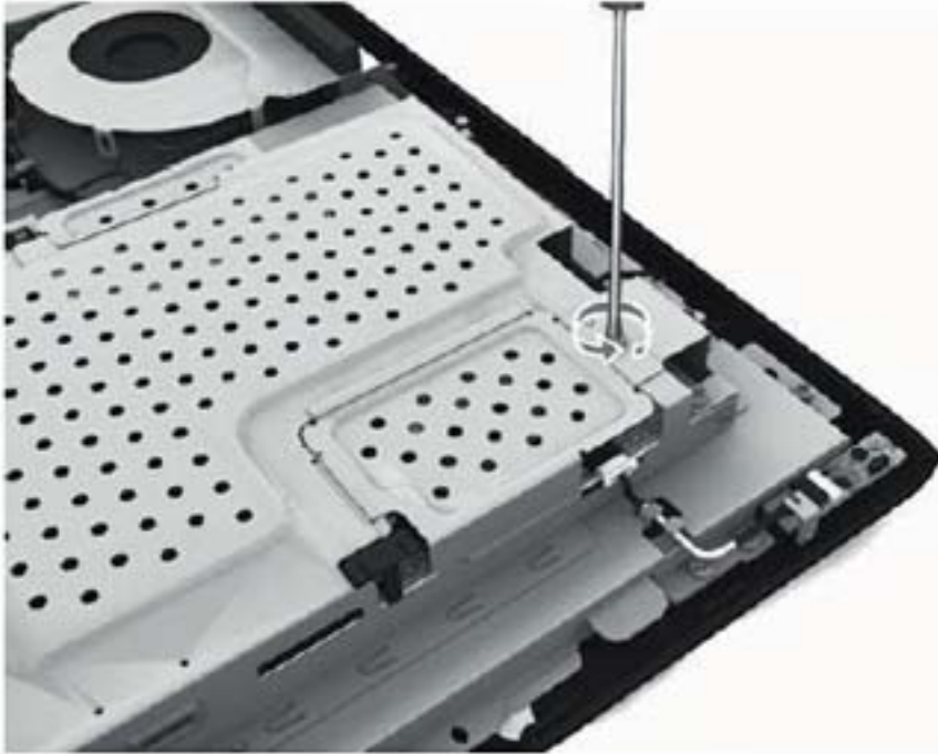
Figure 6-18 Removing the memory cover screw
