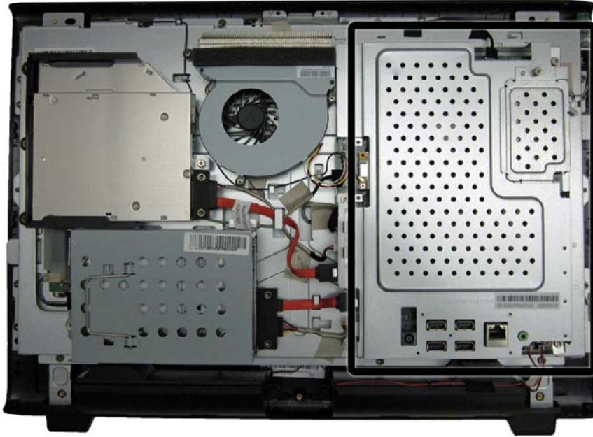
Figure 6-47 System board location
