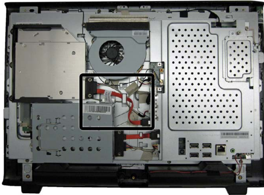
Figure 6-38 Optical drive cable location
