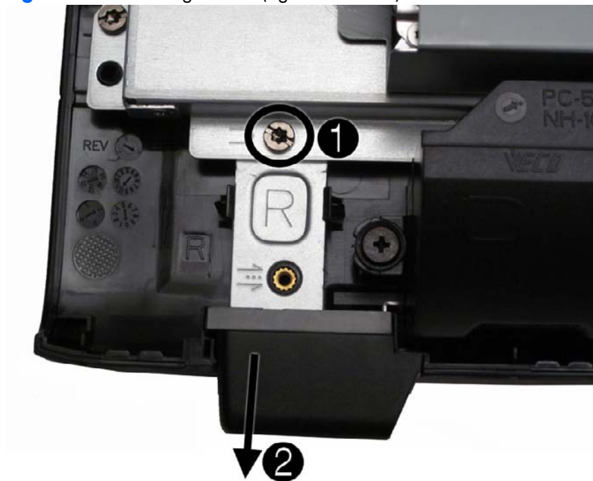
Figure 6-5 Removing the feet (right foot shown)
