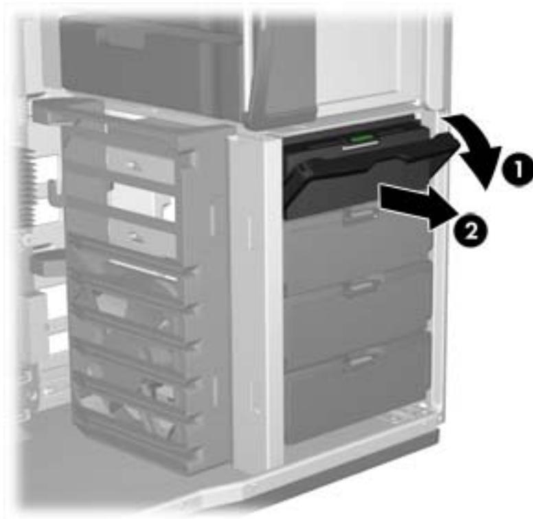
4. Carefully separate the upper hard drive carrier rails (1), tilt the drive outward (2), carefully separate the lower carrier rails (3), and then remove the drive from the carrier, as shown in the following figure.
