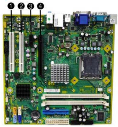
Figure 6-8 Expansion Slot Locations – HP Pro 3120
