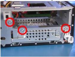
8. Slide the cage down and pull the assembly out of the computer.
