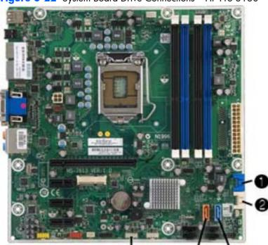
Figure 6-22 System Board Drive Connections – HP Pro 3130
