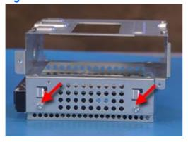
10. Slide the hard drive out of the drive cage assembly.
