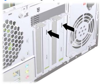
**b.** If you are removing a standard PCI card or PCI Express x1 card, hold the card at each end, and carefully rock it back and forth until the connectors pull free from the socket. Pull the expansion card straight up from the socket then away from the inside of the chassis to release it from the chassis frame. Be sure not to scrape the card against the other components.
