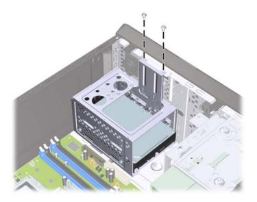
4. Push down the latch on the side of the hard drive cage (1), then slide the hard drive cage away from the bottom of the chassis (2) as shown below.
