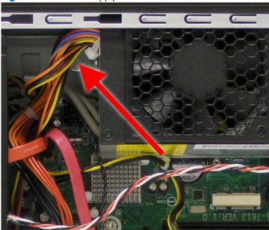
**6.** Pull the power supply toward the front of the chassis, and then lift the power supply up and out of the chassis.
