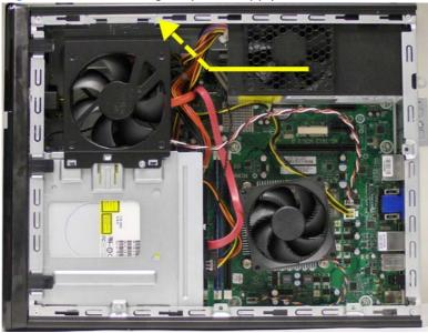
NOTE: If the power supply includes a voltage select switch, make sure to set the red switch to the setting (230 V or 115 V) appropriate for the country in which the computer is used. Spare power supplies normally arrive set for 230 V.
