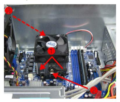
△ **CAUTION:** Heat sink retaining screws should be tightened in diagonally opposite pairs (as in an X) to evenly seat the heat sink to the processor. This is especially important as the pins on the socket are very fragile and any damage to them may require replacing the system board.
