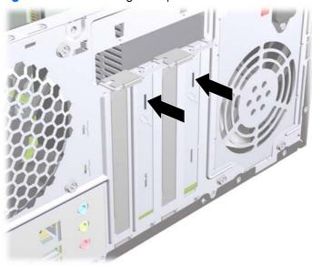
**b.** If you are removing a standard PCI Express x1 card, hold the card at each end, and carefully rock it back and forth until the connectors pull free from the socket. Pull the expansion card straight up from the socket then away from the inside of the chassis to release it from the chassis frame. Be sure not to scrape the card against the other components.
