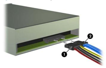
5. Pull out the drive latch and swing it to the left(1), then slide the drive out of the front of the chassis (2).
