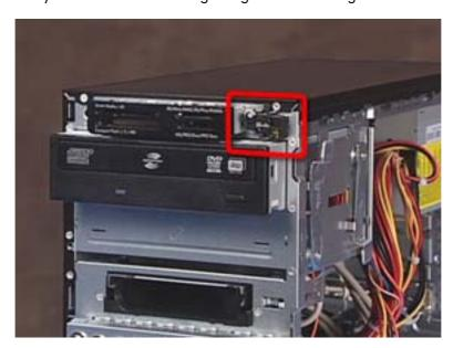
Remove the power switch cable from the clips located in the optical drive bay on the inside of the chassis.
