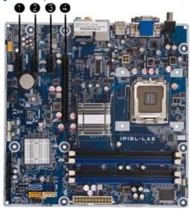
**Figure 5-9** Expansion Slot Locations – HP Pro 3125
