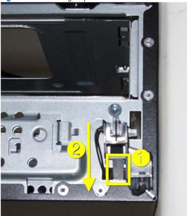
10. Remove the power switch cable from the clips located in the optical drive bay on the inside of the chassis.
