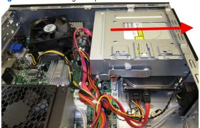
NOTE: To replace the drive, reverse the removal procedure.
