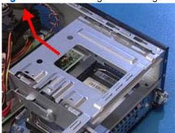
**9.** The hard drive is secured to the drive cage by four screws, two on each side. Remove the screws, and then slide the hard drive out of the drive cage assembly.
