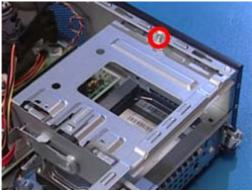
Figure 6-26 Hard drive cage screw location – front
