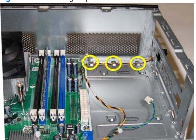
**9.** Press the tab **(1)** on the bottom of the power switch to disengage it from the chassis, slide the switch downward to disengage the tabs from the chassis **(2)**, and then pull the power switch away from the chassis while guiding the wires through the hole in the chassis.
