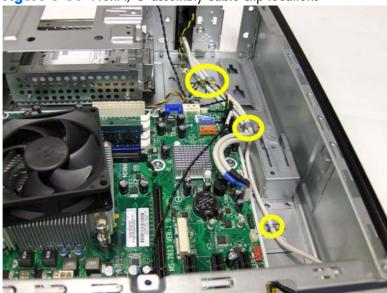
7. Disconnect the hard drive activity LED connector from rest of the power switch cable bundle.
