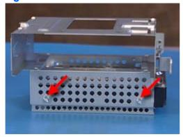
Figure 6-29 Hard drive screws
