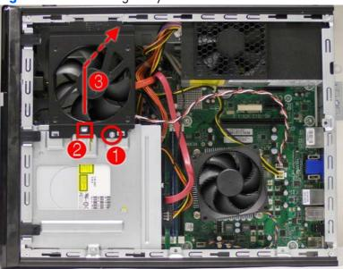
Figure 6-16 Removing the system fan
