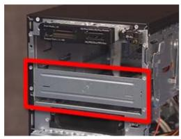
When inserting an optical drive, pull out on the drive latch and insert its peg into the hole marked 2, and then slide the drive back until it locks into position.
