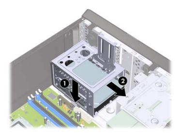
5. Lift the hard drive cage out of the chassis.
