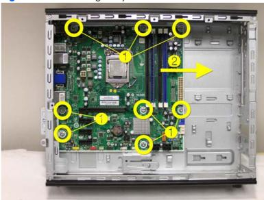
11. Slide the system board toward the front of the chassis, and then lift the board out of the computer (2).
