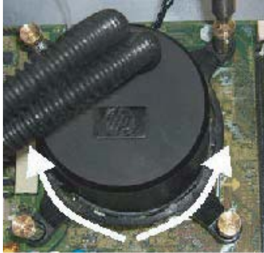
Figure 5-59 Positioning the LCS cold plate
