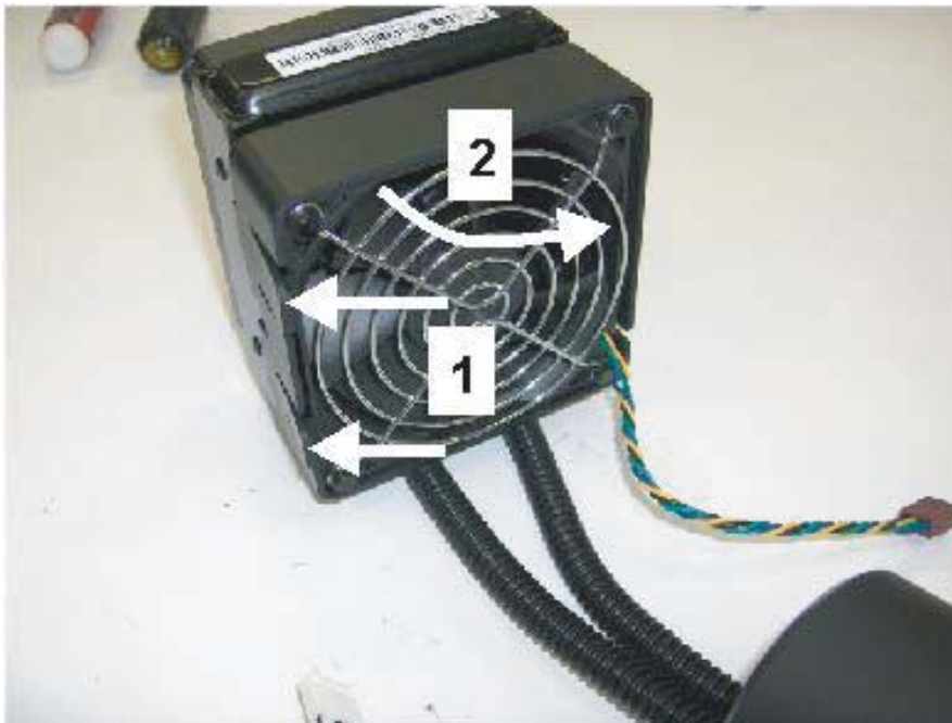
Figure 5-55 Removing the rear system fan from the radiator fan holder
