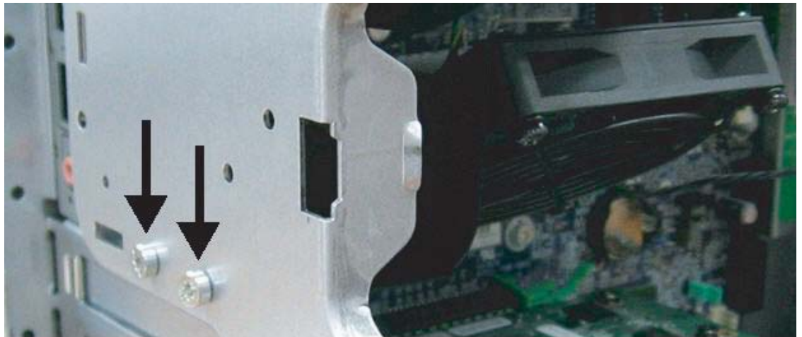
Figure 5-66 Fastening the LCS VR fan
