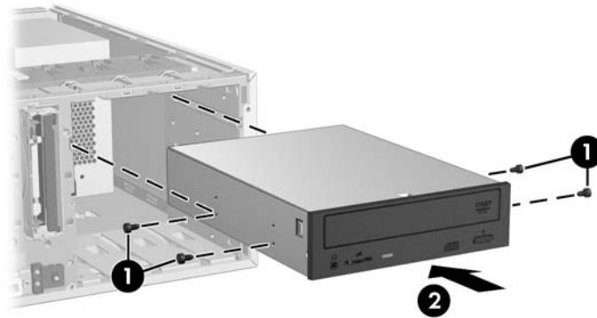
Figure 5-20 Installing the optical drive
