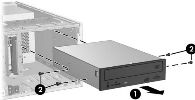
Figure 5-19 Removing the optical drive screws
