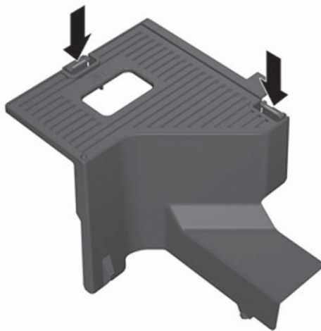
Figure 5-26 Removing the airflow guide
