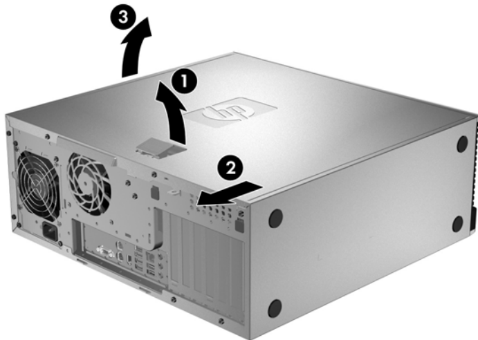
Figure 5-4 Removing the side access panel
