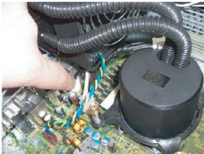
Figure 5-52 Disconnecting the LCS pump cable
