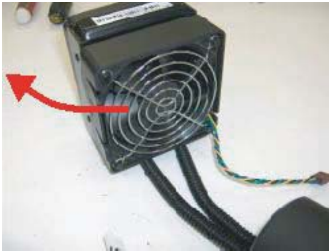
Figure 5-56 Installing the system fan in the LCS radiator fan holder
