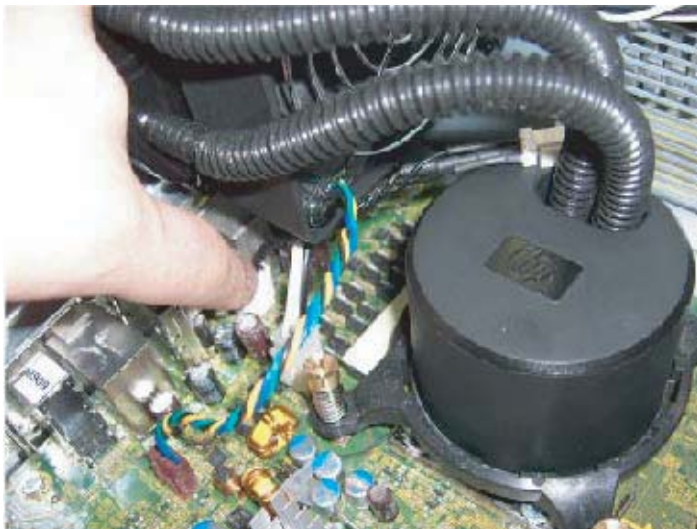
Figure 5-61 Connecting the LCS pump cable
