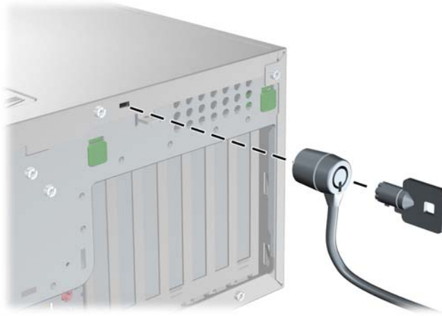
Figure 5-3 Removing the cable lock
