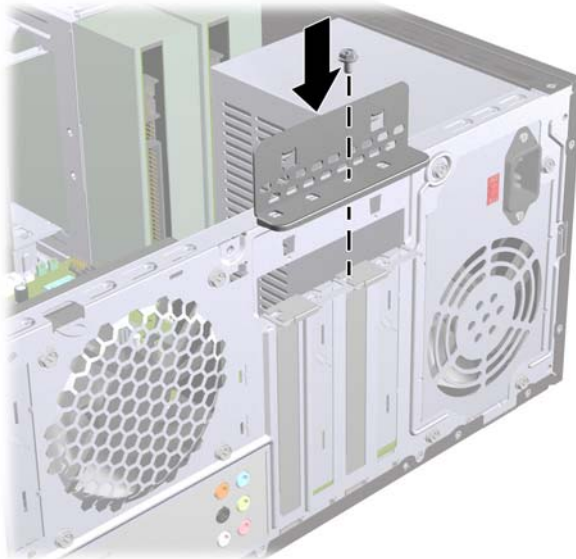
Figure 7-13 Securing the Expansion Cards and Slot Covers
