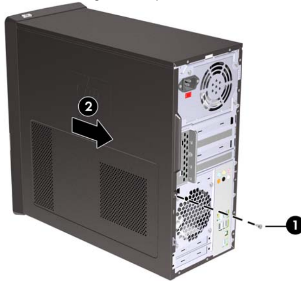
Figure 7-2 Removing the Computer Access Panel
