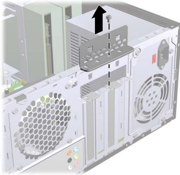
Figure 7-8 Opening the Slot Cover Lock
