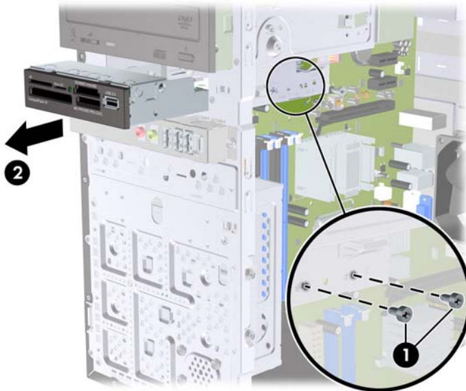
Figure 7-22 Removing a 3.5-inch Device (Media Card Reader Shown)
