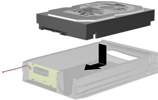
7. Replace the four screws in the bottom of the carrier to hold the drive securely in place.
