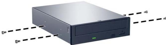
9. Position the guide screws on the drive into the J-slots in the drive bay. Then slide the drive toward the front of the computer until it locks into place.
