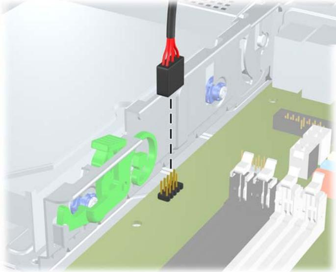
**Figure 2-30** Disconnecting the Media Card Reader 1394 Cable
