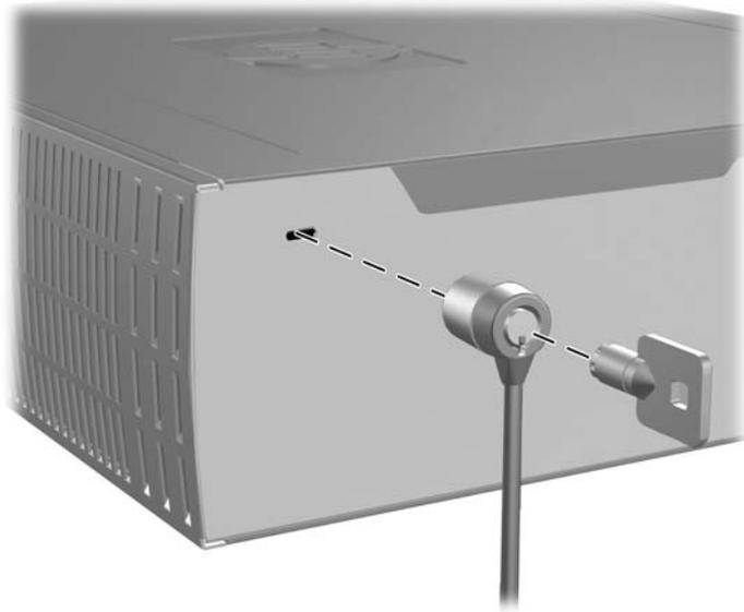
**Figure 2-13** Installing a Security Lock
