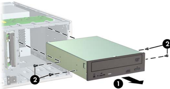
Figure 4-38 Removing the optical drive screws
