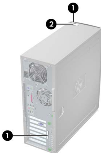
Figure 1-4 Serial number and COA label location
