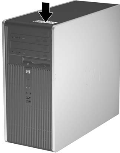
Figure 1-2 Serial Number and Product ID Location
