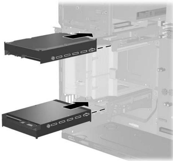
Figure 2-27 Sliding a Hard Drive into the Drive Bay
