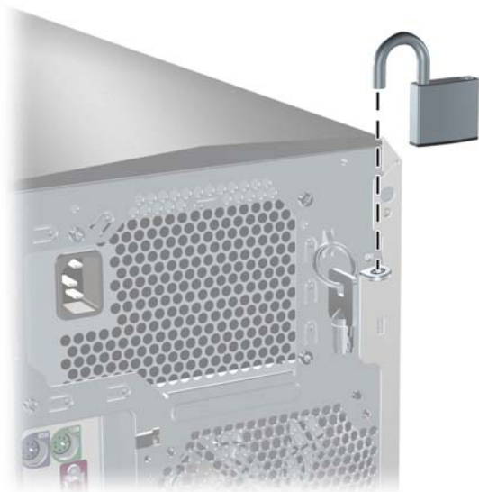
Figure 4-3 Removing the security lock
