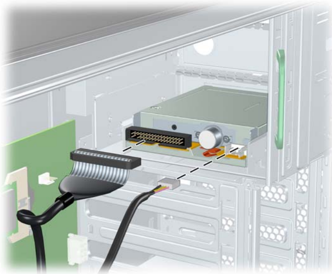
Figure 4-32 Disconnecting cables from the diskette drive
