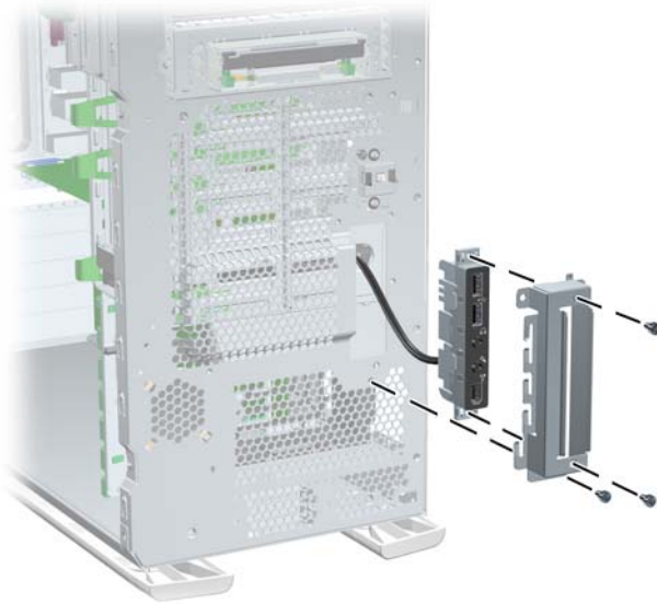
Figure 4-9 Removing the front panel I/O device assembly
