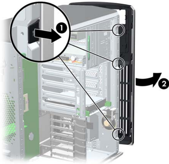
Figure 4-6 Opening the front bezel
