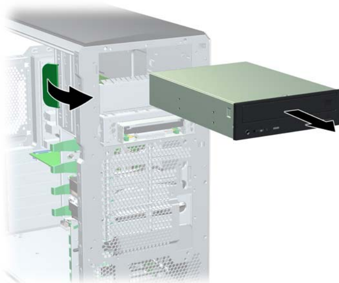
Figure 4-29 Removing the optical drive from the chassis
