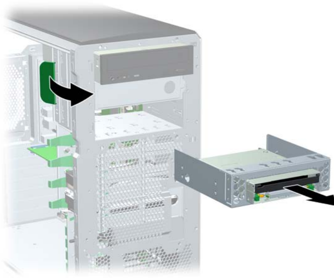
Figure 4-33 Removing the diskette drive from the chassis
