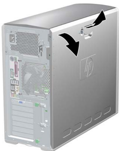
Figure 4-5 Opening the access panel
