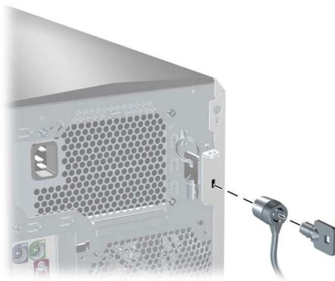
Figure 4-4 Removing the cable lock
