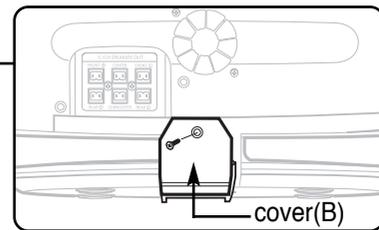
**3** Put the speaker cable connected to the Speaker OUT port into the left groove.
