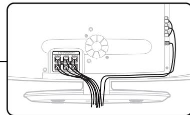
**4** Put the cables connected to the Video OUT, Component OUT and Audio IN ports into the right groove.
