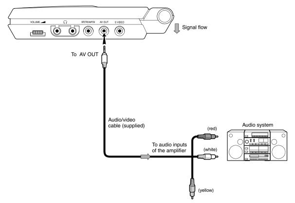
When the AV OUT or BITSTREAM/PCM jacks are connected to the audio input terminals of an audio system, sounds of discs can be heard on the connected audio system. For instructions on connections to audio systems, see also page 57.
