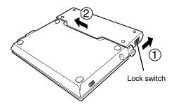
5 Replace the connector cover on the bottom of the player.
