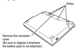
4 Turn the battery pack over and insert four catches into the player's corresponding holes. Then, slide the battery pack in the direction of the arrow ② until a "click" is heard.
