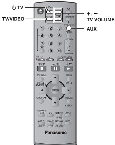
You can use the remote control to operate a Panasonic television. Connect your equipment referring to “Cable TV box or video cassette recorder connection” (→ page 7).
