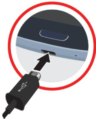
1. Plug the flat end of the Travel Charger into the charging/USB port and the other end into a standard AC wall outlet.
