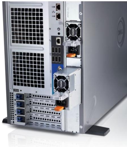
The PowerEdge T620 supports up to two AC or DC power supplies with 1 + 1 redundancy, auto-sensing, and auto-switching capability.
