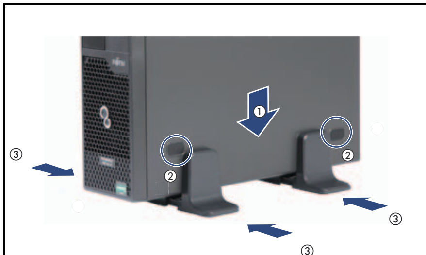
Figure 4: Placing the server on stabilizers
