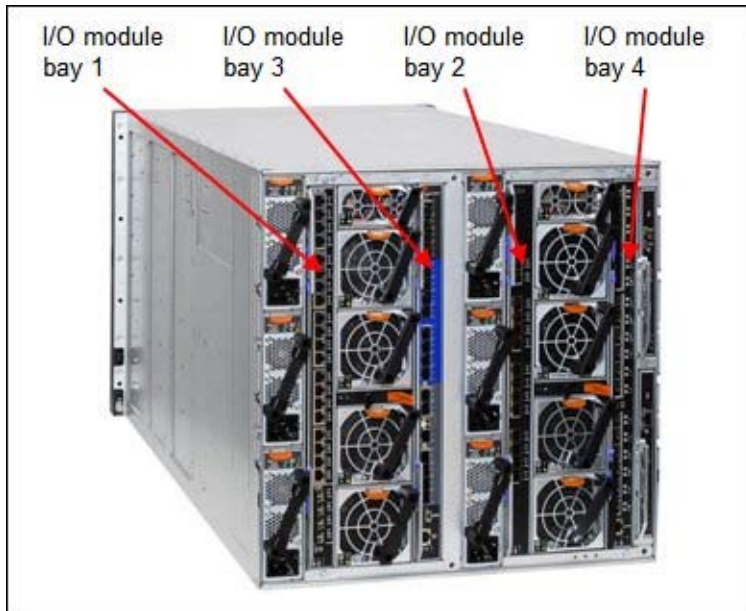
Figure 6. Location of the switch bays in the IBM Flex System Enterprise Chassis
