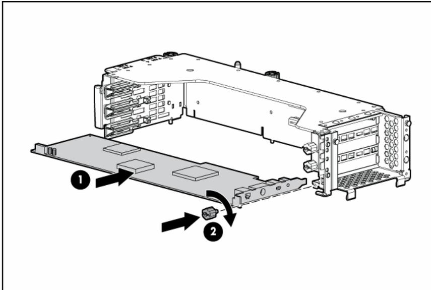
8. Lock the PCI retaining clip.
