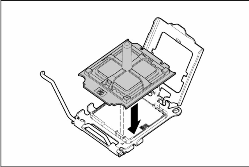
10. Press down firmly until the processor installation tool clicks and separates from the processor, and then remove the processor installation tool.
