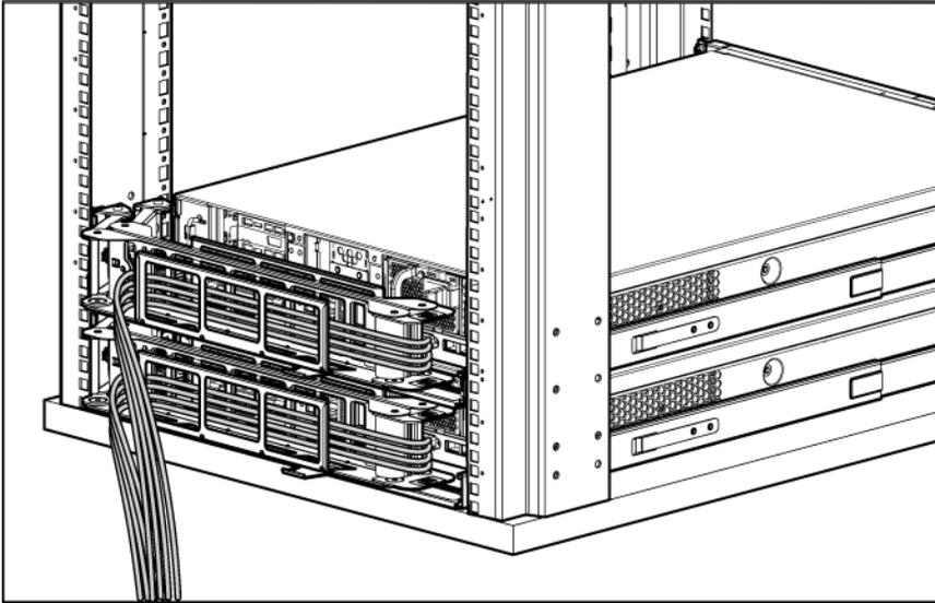
6. Connect the power cord to the AC power source.
