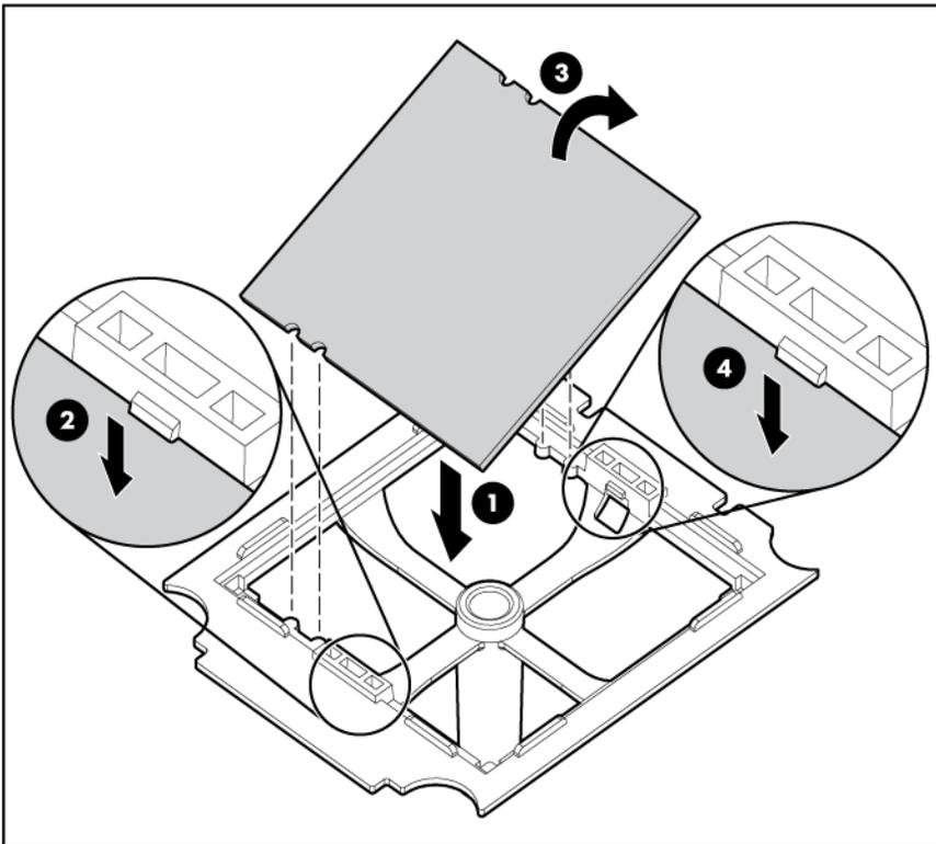
9. Align the processor installation tool with the socket and install the processor.
