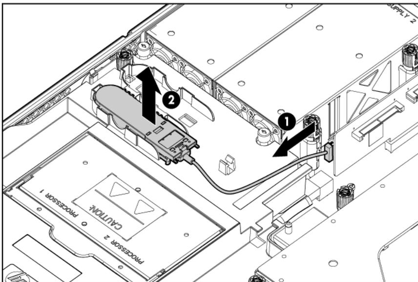
5. Remove the air baffle.
