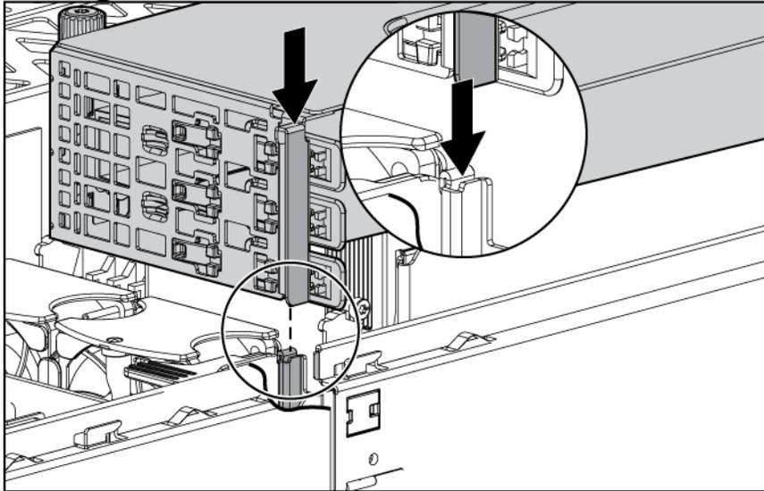
2. Tighten the thumbscrews to secure the PCI riser cage:
