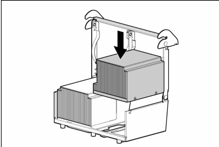
14. Close the heatsink retaining bracket.
