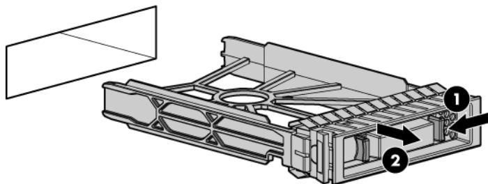
To replace the blank, slide the blank into the bay until it locks into place.
