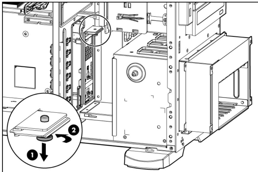
9. Remove the PCI-X expansion cage.
