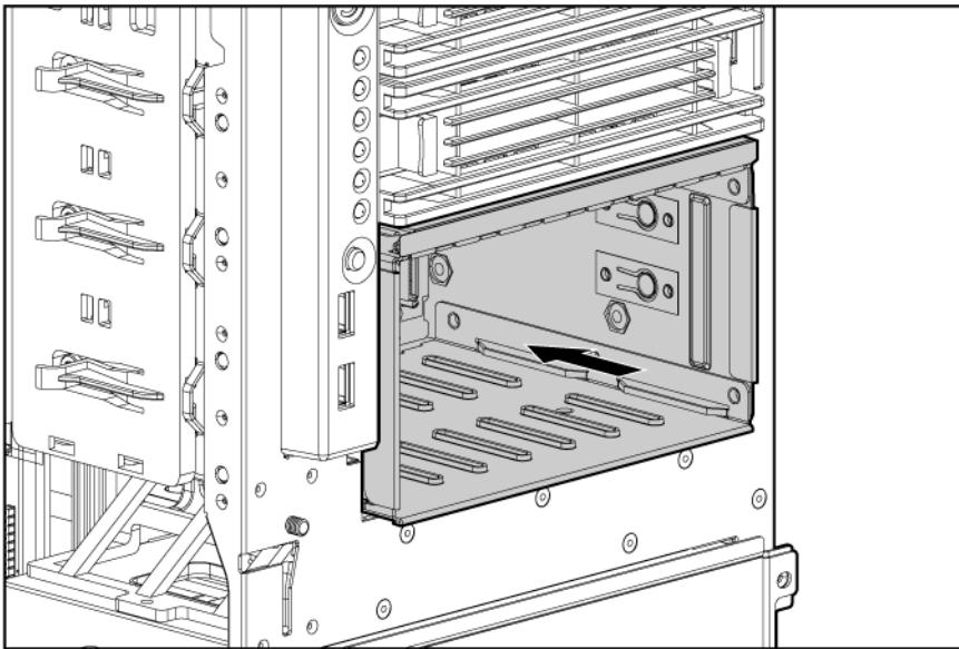
3. Connect all cables to the spare hard drive cage.
