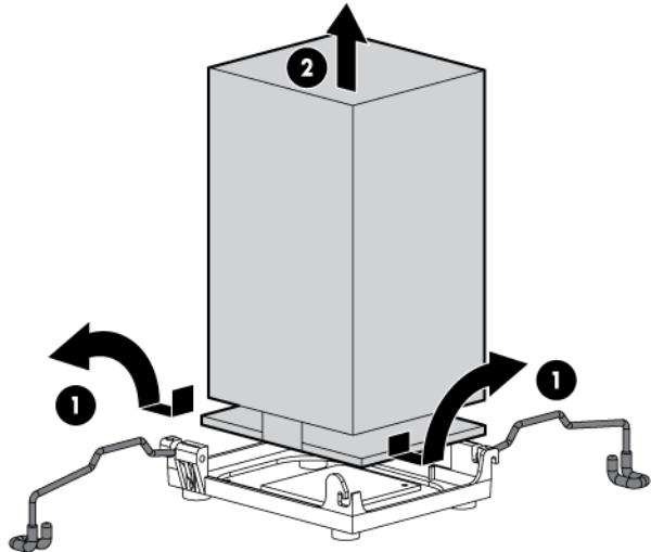
7. Open the processor retaining latch and the processor socket retaining bracket.
