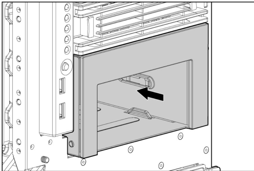
2. Connect all cables to the spare hard drive cage.
