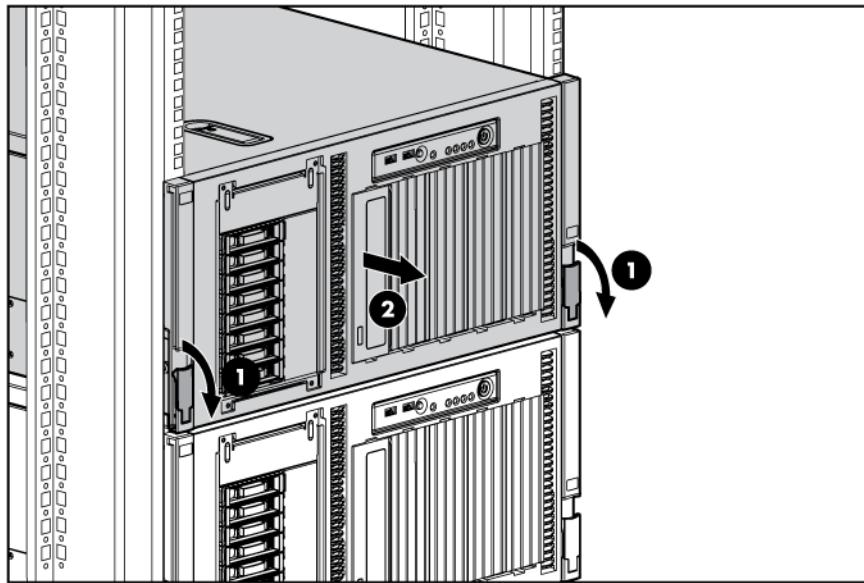
4. After performing the installation or maintenance procedure, press the rail-release latches and slide the server back into the rack.
