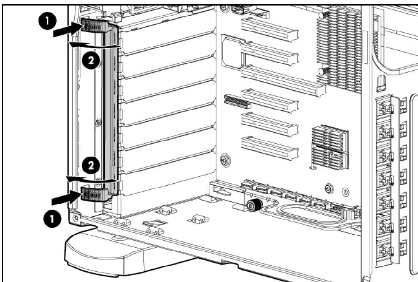
4. Remove the expansion slot cover.
