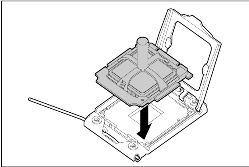
3. Press down firmly until the processor installation tool clicks and separates from the processor, and then remove the processor installation tool.
