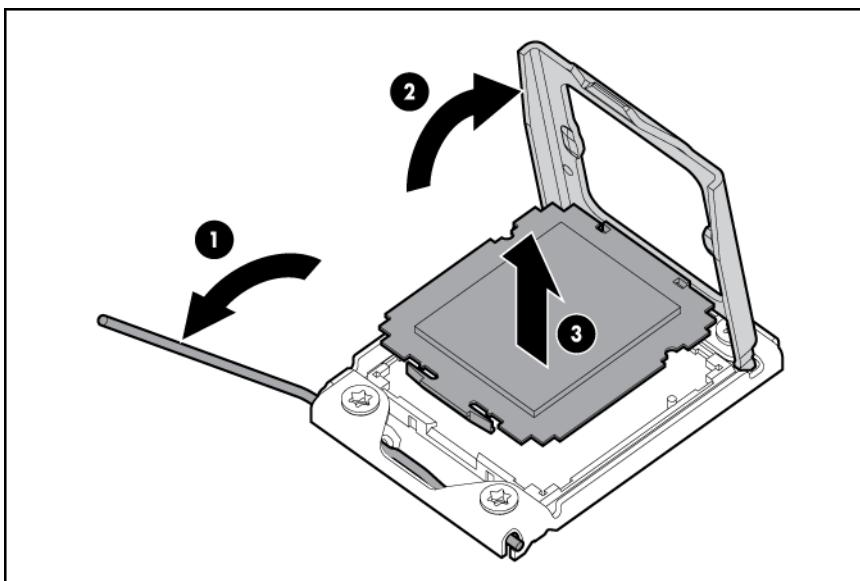
3. Install the processor socket cover onto the processor socket of the failed system board.
