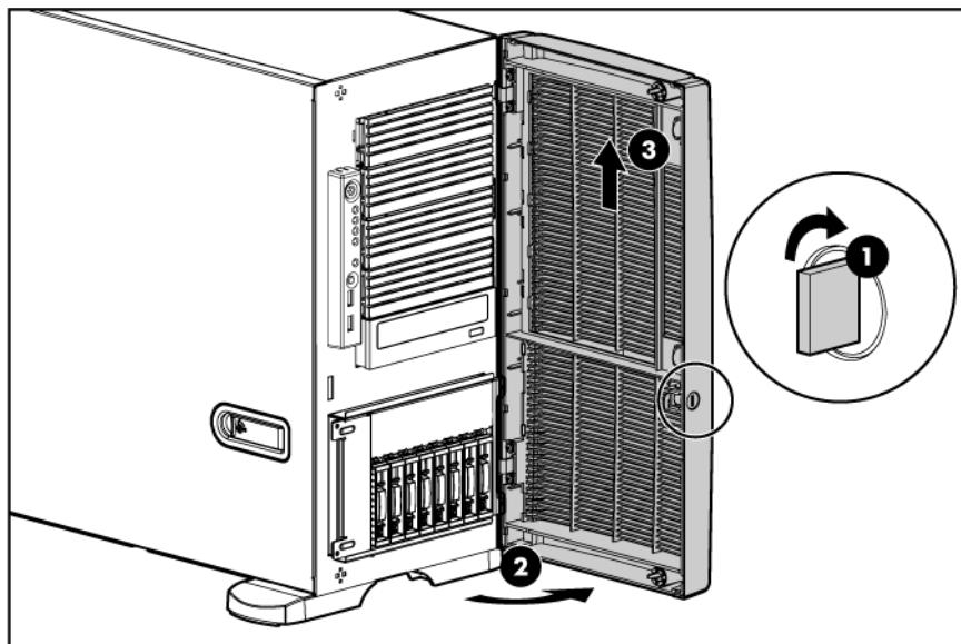
For operations involving removable media bay access, the media bay panel can be removed from the bezel.
