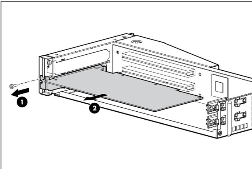
To replace the components, reverse the removal procedure.
