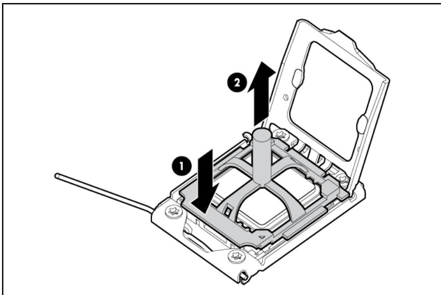
4. Close the processor retaining latch and the processor socket retaining bracket.
