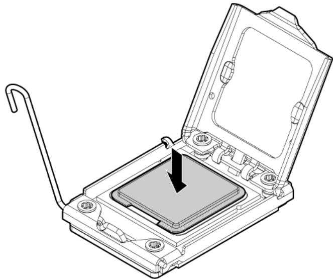
5. Close the processor retaining latch and the processor socket retaining bracket.
