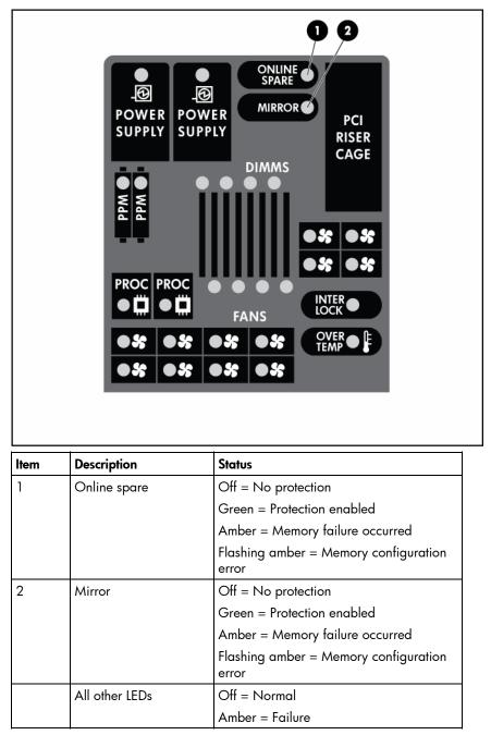
**IMPORTANT:** If more than one FBDIMM slot LED is illuminated, further troubleshooting is required. Test each bank of FBDIMMs by removing all other FBDIMMs. Isolate the failed FBDIMM by replacing each FBDIMM in a bank with a known working FBDIMM.
