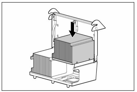
**13.** Close the heatsink retaining bracket.
