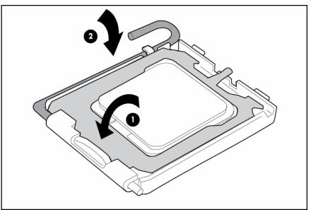
△ **CAUTION:** To prevent possible server malfunction or damage to the equipment, be sure to completely close the processor locking lever.
