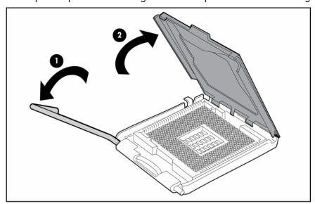
5. Open the processor retaining latch and the processor socket retaining bracket.
