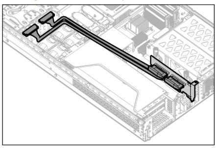
PCI SAS cabling to optional expansion board controller
