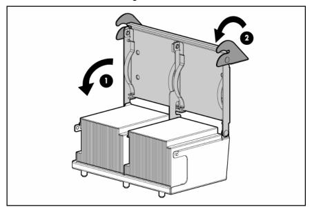
**14.** Open the latches on the corresponding PPM slot.
