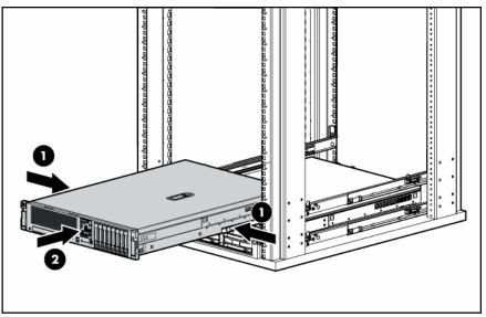
**b.** Press the server firmly into the rack to secure it in place.
