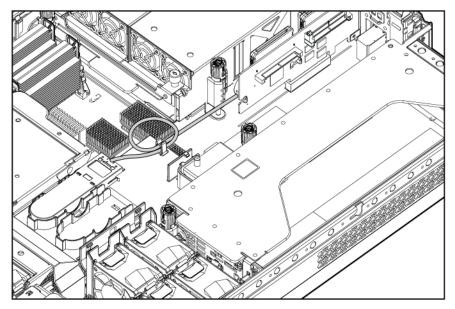
**NOTE:** Use the retaining clip to manage excess cable slack.
