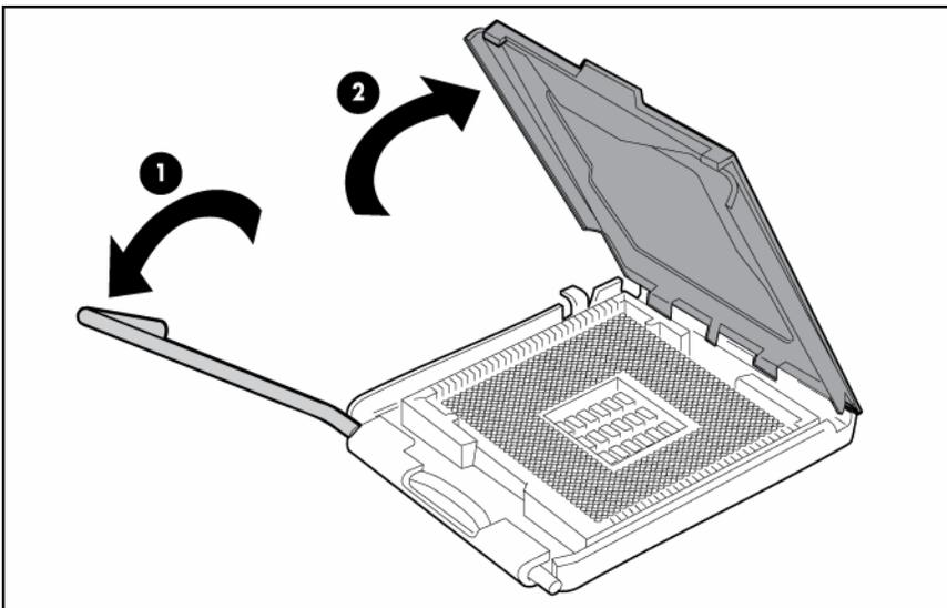
6. Remove the processor socket protective cover.
