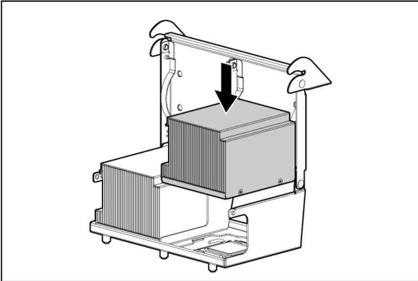
**13.** Close the heatsink retaining bracket.
