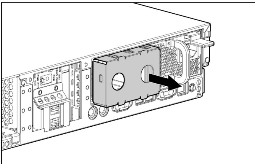
3. Slide the power supply into the power supply bay.
