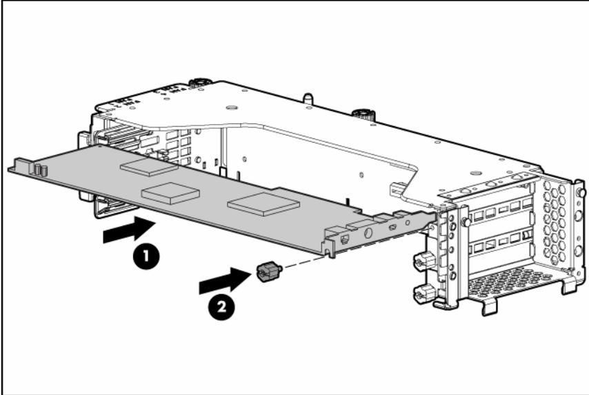
8. Lock the PCI retaining clip.
