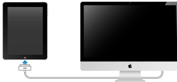
**Important:** The iPad battery may drain instead of charge if iPad is connected to a PC, to a computer that's turned off or is in sleep or standby mode, to a USB hub, or to the USB port on a keyboard.
