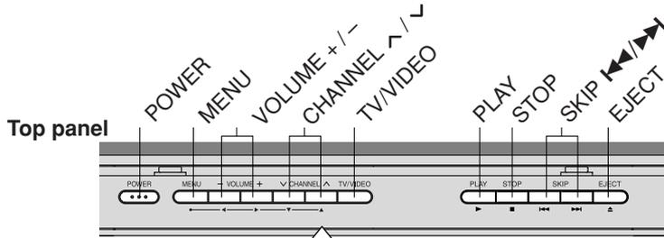
The volume and channel buttons on the top panel can be used as ▲/▼ and ◀▶ buttons while the TV menu is displayed on screen.
