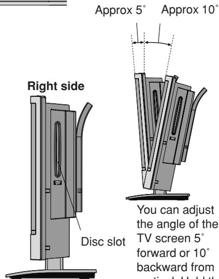
You can adjust the angle of the TV screen 5° forward or 10° backward from vertical. Hold the base of the TV/DVD while adjusting the angle.
