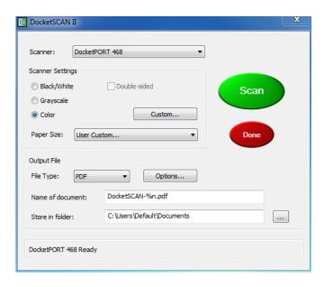
The second way is through the TWAIN control panel, which you can find by pressing the "<u>Custom...</u>" button on the DocketSCAN II<sup>®</sup> control panel. The TWAIN control panel (shown below) allows you to control all details and settings of the scanner. This type of "fine-adjustment" of your scans may be required for some of your document needs.
