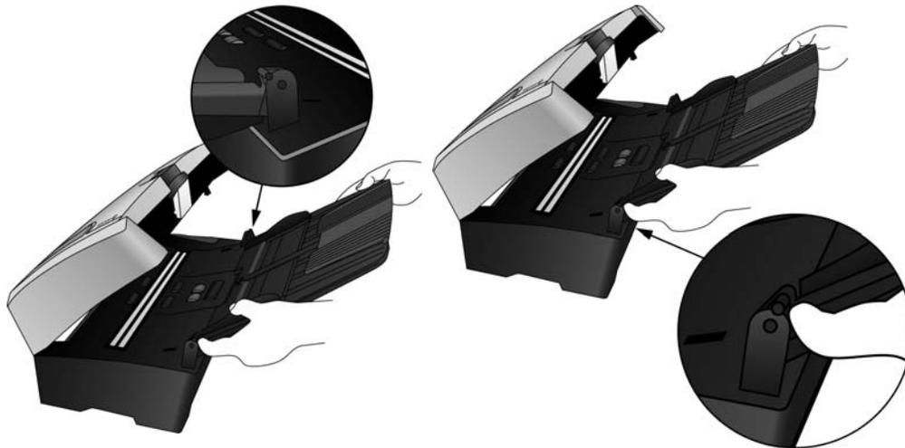
5. Insert the short pins on each side of the output tray into the holes on the scanner.
