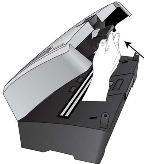
3. Press on the roller housing until it snaps into place in the scanner lid.
