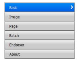
Configure the scan settings or check the version information. When you select [Basic], [Image], [Page], [Batch] or [Endorser], the details are displayed on the right side. When you select [About], the version information of the PaperStream IP driver is displayed.
