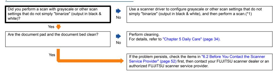
\*1: The scanned image may differ from the original image significantly if you simply "binarize" (output in black & white) a picture or a photo. If possible, use a scanner driver to configure grayscale or other scan settings that do not simply "binarize" (output in black & white), and then perform a scan.
