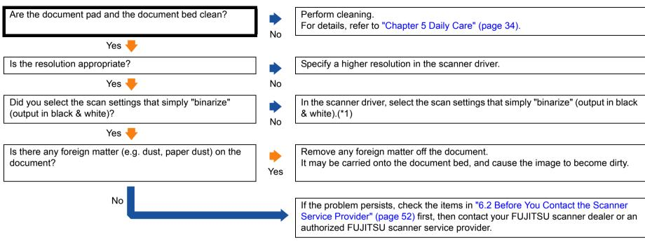
\*1: When scanning in grayscale or color, the scanned image may not become sharp and clear. If possible, use a scanner driver to configure the scan settings that simply "binarize" (output in black & white), and then perform a scan.
