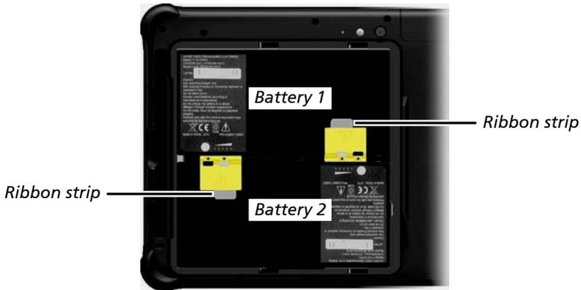
3. Fit another battery pack into place. Note the orientation of the battery pack. Hold the battery pack at an angle and insert its small tabs to the corresponding notches in the battery compartment. Then, lift the yellow protection sheet in the battery compartment and plug the battery connector.
