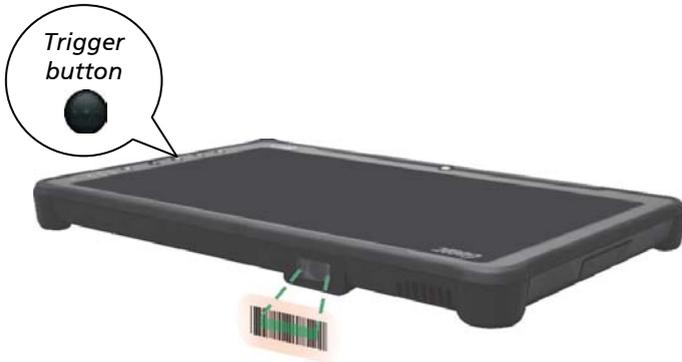
**NOTE:** If the code being scanned is highly reflective (e.g., laminated), it may be necessary to tilt the code +5° to prevent unwanted reflection.
