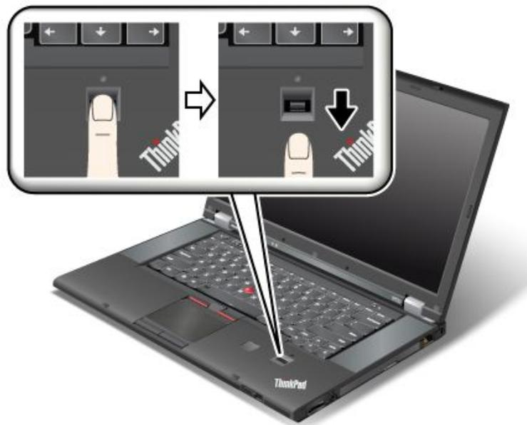
To swipe your finger over the reader, place the ball of your finger, that is, the central part of the fingerprint, on the small circle above the reader. Make sure that the entire top joint of the finger is on the reader. Then Apply light pressure and swipe your finger across the reader in one smooth motion.
