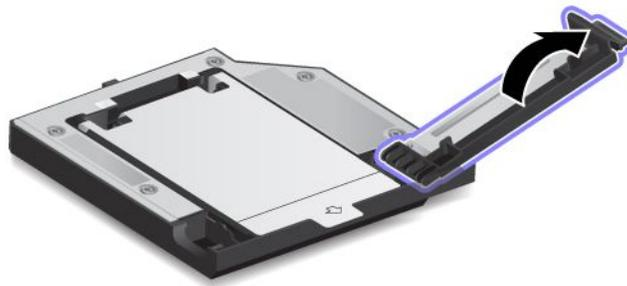
3. Lift up the cover film and insert the hard disk drive with the label facing upward.
