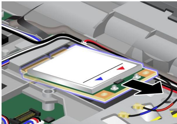
8. Align the contact edge of the new wireless WAN card with the corresponding socket.
