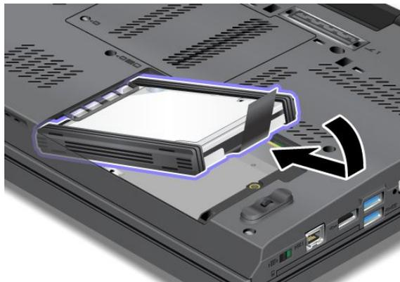
9. Slide the hard disk drive or solid state drive firmly into place.
