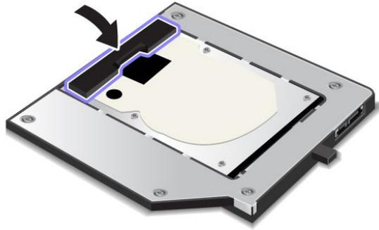
6. Insert the ThinkPad Serial Hard Drive Bay Adapter III into the Serial Ultrabay Enhanced bay.
