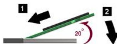
8. Pivot the memory module downward until it snaps into place.
