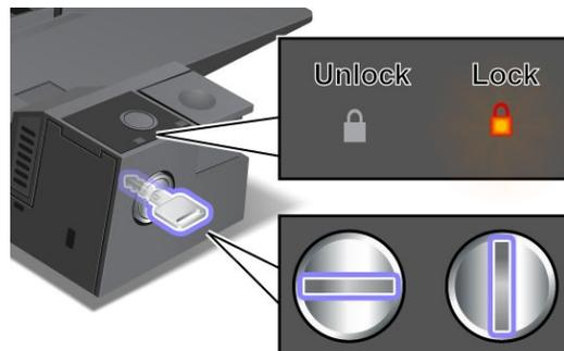
When the key is in the locked position, the eject button of the docking station is locked, and you cannot remove your computer. The key lock indicator lights when the eject button is locked.
