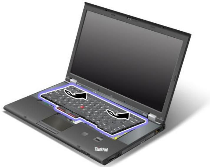
3. Push down the keyboard firmly and then slide the keyboard in the direction shown by the arrows.
