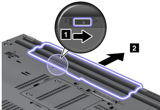
4. Slide the new battery into the computer.
