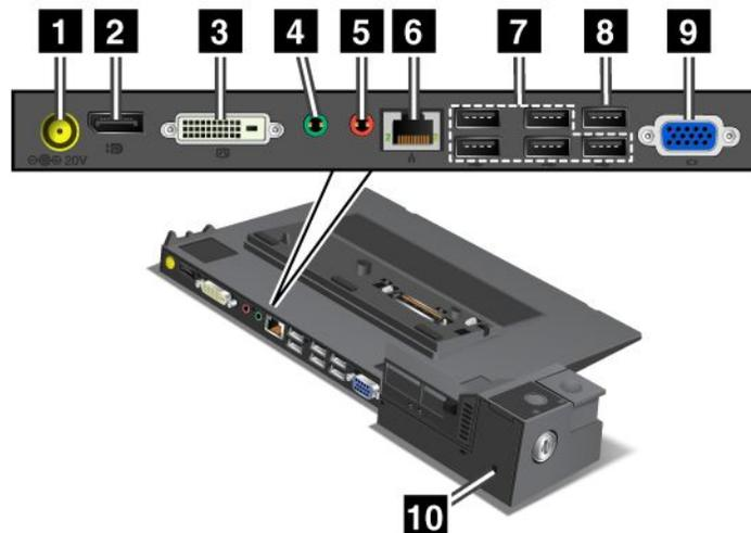
**1 Power jack:** Connect the ac power adapter.
