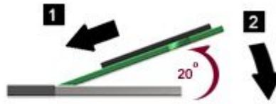
8. Pivot the memory module downward until it snaps into place.
