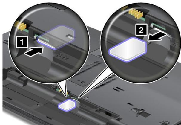
5. Hold the new card with the metal contact facing upward, and insert the card firmly into the slot until you hear a click.
