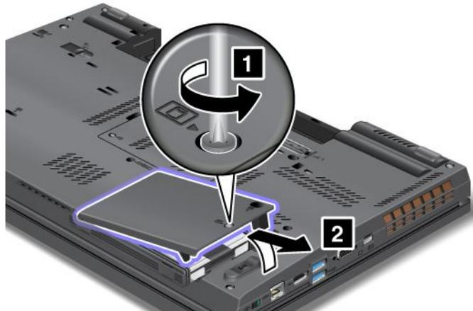
5. Remove the hard disk drive or solid state drive by pulling out the tab.
