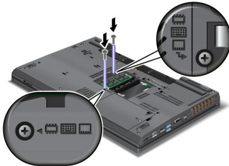
5. Reinstall the memory slot cover back in place.
