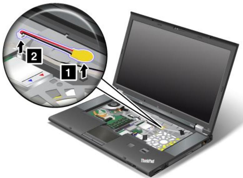
6. Install the new backup battery and attach the connector .
