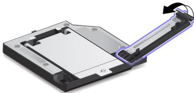
6. Insert the ThinkPad 12.7 mm Serial ATA Hard Drive Bay Adapter III into the Serial Ultrabay Enhanced bay.
