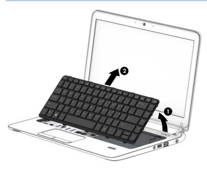
6. Rotate the keyboard until it rests on the palm rest (1).
