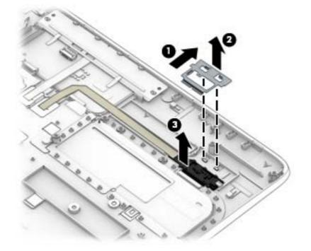
Reverse this procedure to install the fingerprint reader assembly.
