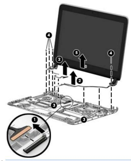
**CAUTION:** When installing the display assembly, be sure that the wireless antenna cables are routed and arranged properly.
