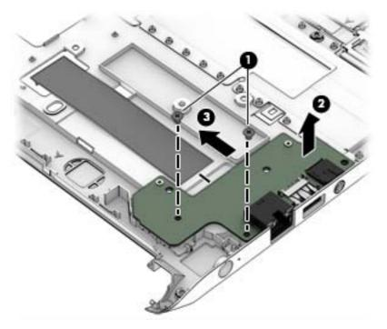
5. Remove the I/O board from the top cover.
