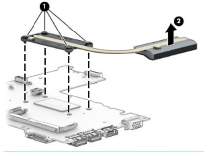
**NOTE:** Thoroughly clean thermal material from the surfaces of the system board component **(1)** and the heat sink **(2)** each time you remove the heat sink. All heat sink and processor spare part kits include thermal material.
