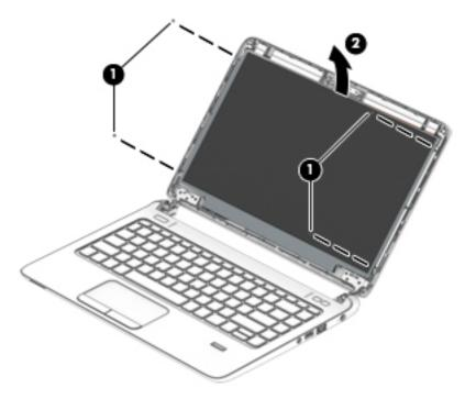
7. Rotate the display panel all the way over (1), disconnect the display cable from the rear of the panel (2), and then remove the display panel (3) from the enclosure.
