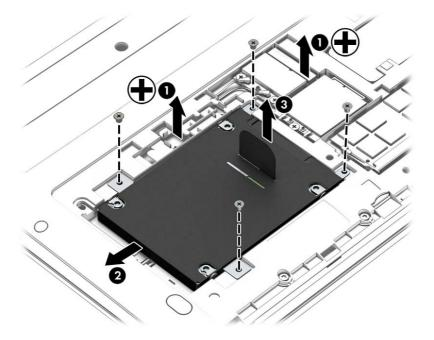
4. To remove the hard drive cover from the hard drive, remove the 4 Phillips PM3.0×3.0 screws (1) that secure the cover to the drive, and then lift the cover off the drive (2).
