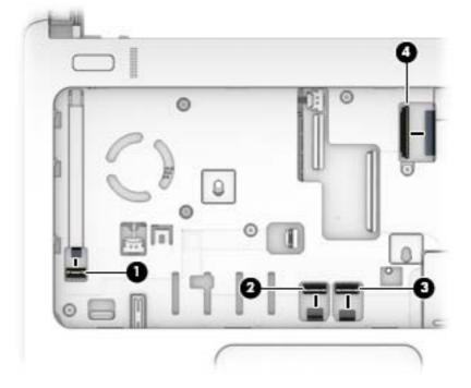
7. Pry the top cover off the computer to disengage it. Lift the top of the top cover (1), and the lift the top cover up and remove it from the computer (2).
