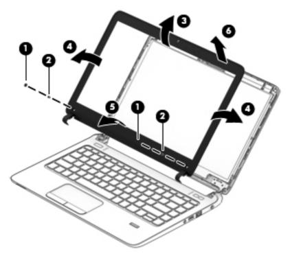
5. If it is necessary to replace the webcam or microphone module, note that cable connects through the hole in the ledge (1) on the display enclosure. Disconnect the cable from the module (2), and then gently pull the module away from the double-sided tape on the display enclosure (3).
