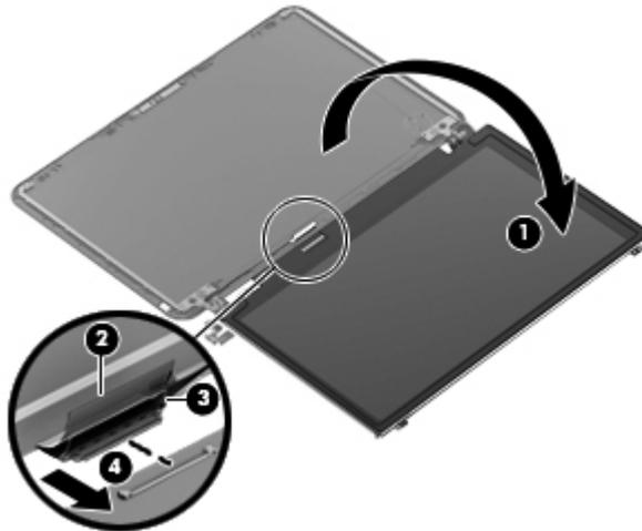
5. If it is necessary to replace the webcam/microphone module:
