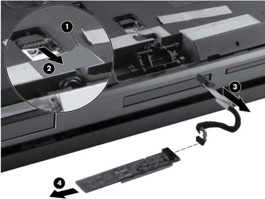
Reverse this procedure to install the Bluetooth module.
