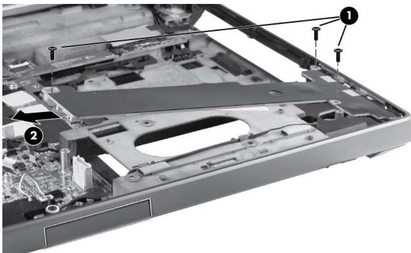
Reverse this procedure to install the audio/USB 3.0 board.
