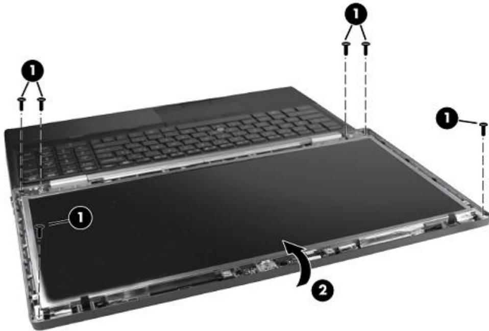
3. Disengage the display panel from the base enclosure by closing the display enclosure to 45 degrees while holding the sides of the display panel.
