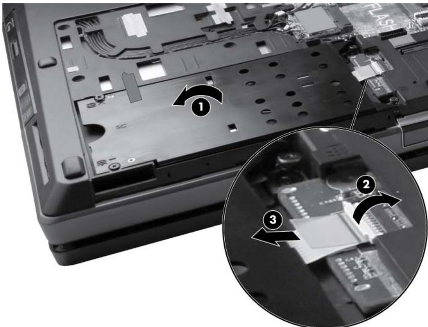
3. Reopen the door, tilt the door towards you **(1)**, and then lift the smart card reader door straight up from the computer **(2)**.
