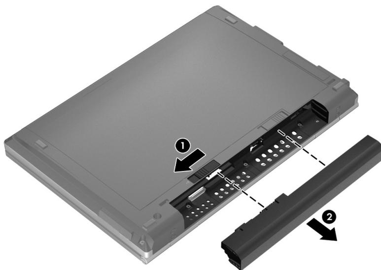
Install the battery by inserting it into the battery bay until you hear a click. The battery release latch automatically resets when the battery is installed.
