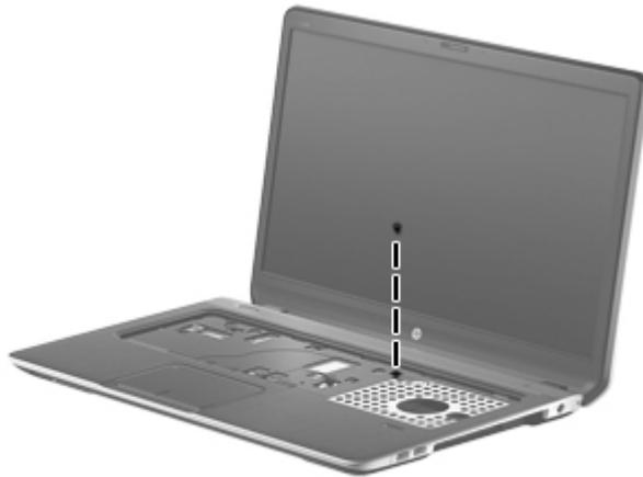
7. Lift the rear edge of the top cover (1) until the left and right sides have disengaged from the base enclosure.
