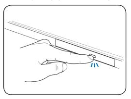
2. Gently pull the drive's front panel to slide the tray out completely. Be careful not to touch the optical drive lens and other mechanisms. Ensure that there are no objects that may get jammed under the drive's tray.
