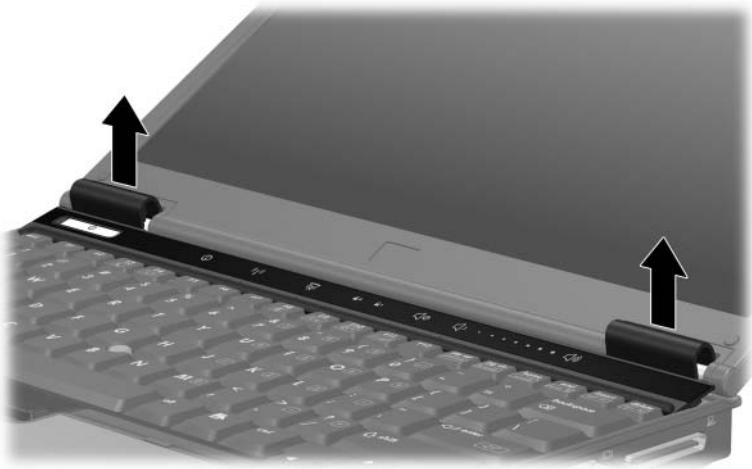
Releasing the Switch Cover, Part 2
