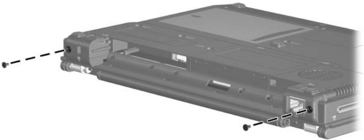
Removing the Display Assembly Screws
