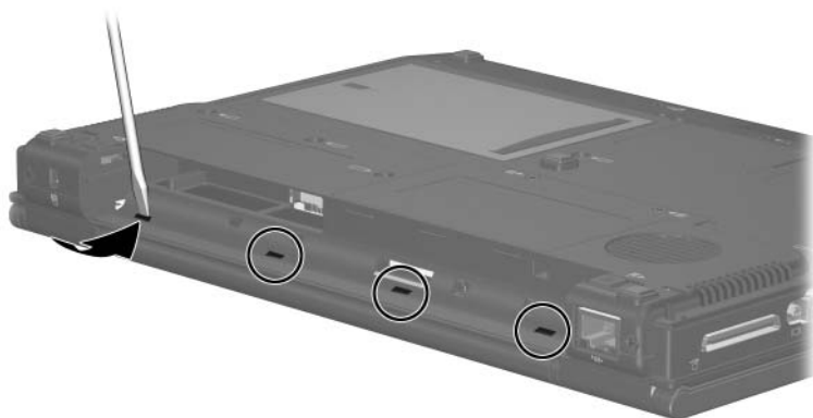
Releasing the Switch Cover, Part 1
