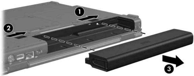
*Removing the Battery Pack*
