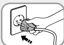
**Plug the power cord firmly into the power outlet and AC adapter.**
