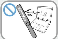
**Avoid exposing a drive to magnetic fields. Security devices with magnetic fields include airport walk-through devices and security wands.**
