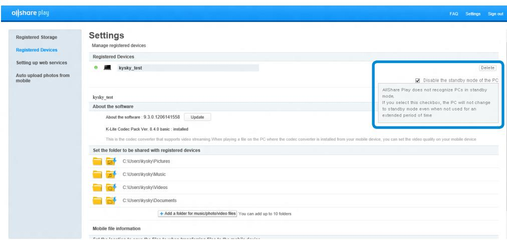
The screenshot shows the 'Registered Devices' section of the AllShare Play Settings. It lists a device named 'kysky\_test'. A callout box highlights the 'Disable the standby mode of the PC' checkbox, which is checked. The tooltip for this checkbox states: 'AllShare Play does not recognize PCs in standby mode. If you select this checkbox, the PC will not change to standby mode even when not used for an extended period of time.'
