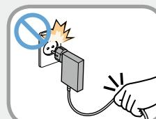
**Unplug the wall-mount AC adapter (adapter and plug intergrated type) from the wall outlet while holding the body and pulling it in the direction of the arrow.**
