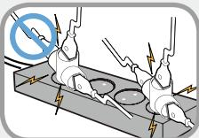
**Do not exceed the standard capacity (voltage/current) of a multiplug or power outlet extension when using it for the product.**
