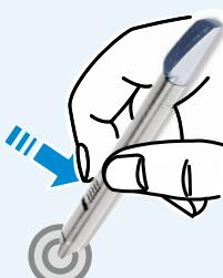
If you press the pen button when the S Pen tip is on the screen, circles appear around the pointer on the screen. Touch the screen with the S Pen while holding down the pen button.
