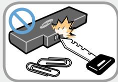
**Take care not to allow metal objects such as a key or clip to touch the battery terminal (metal parts).**
