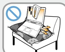
**Avoid blocking the vent at the bottom or side of the computer when using it on a bed or cushion.**
