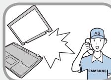
**If the computer is broken or dropped, disconnect the power cord and contact a service center for a safety check.**
