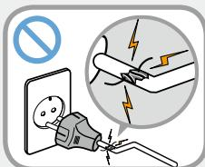
**Do not use a damaged or loose main plug or power cord or power outlet.**
