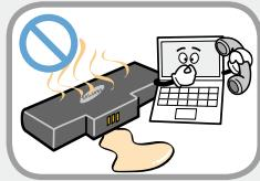
**If liquid leaks out of the product(or battery) or there is a funny smell coming from the product(or battery), remove the the product(or battery) the computer and contact a service center.**
