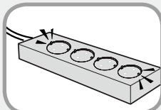
**Connect the power cord to an outlet or multiple power plug (extended cable) with a ground terminal.**
