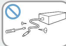
**Never disassemble the power supply or AC adapter.**
