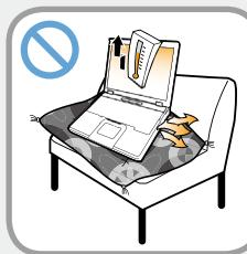
**Do not use the computer in a badly ventilated location such as on bedding, on a pillow or cushion, etc, and do not use it in a location such as room with floor heating as it may cause the computer to overheat.**
