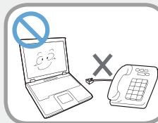
**Do not connect a phone line connected to a digital phone to the modem.**
