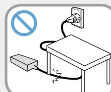
**Do not place heavy objects or step onto the power cord or AC adapter to avoid damaging the power cord or AC adapter.**
