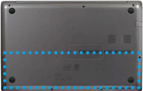
The location of the internal battery
