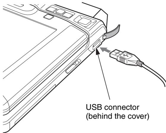
**Figure 32. Connecting USB to System**
