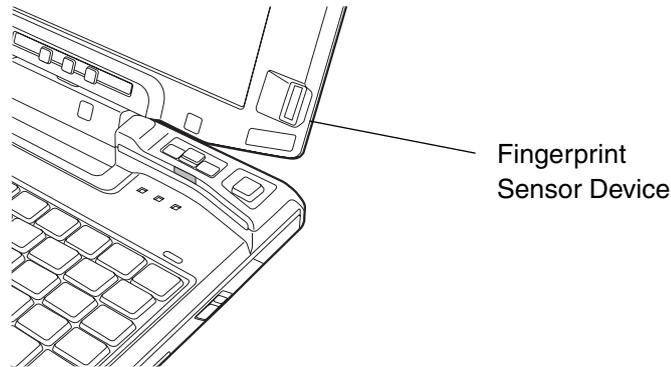
**Figure 42. Fingerprint sensor**
