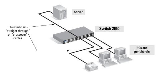
The Switch 2650 is designed to be used primarily as a desktop switch to which end nodes, printers and other peripherals, and servers are directly connected, as shown in the above illustration. Notice that the end node devices are connected to the switch by "straight-through" or "crossover" twisted-pair cables. Either cable type can be used because of the "HP Auto-MDIX" and "IEEE Auto MDI/MDI-X" features on the Switch 2650.
