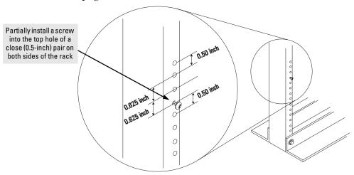
3. Place the switch in the rack and lower it so the notches in the bottom of the bracket slide onto the screws, then tighten these screws.
