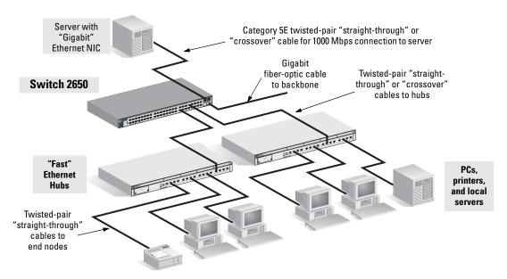
The Switch 2650 also works well as a segment switch. That is, with its high performance, it can be used for interconnecting network segments—simply connect the network hubs that form those segments to the switch, or you can also connect other switches.
