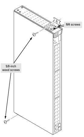
Note that the brackets are attached on opposite corners. This improves the stability of the switch on the wall.
