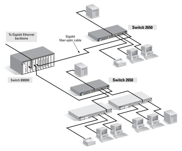
The simpler desktop and segment networks shown in the previous two examples can easily be combined and expanded. For example, you could use an HP Procurve Switch 8000M to interconnect each of your smaller switched workgroups to form a larger switched network. All the devices in this network can communicate with each other. With a Gigabit-SX Module, for example, in the Switch 8000M, the entire switched topology could be connected to a campus backbone, as shown in the illustration above.
