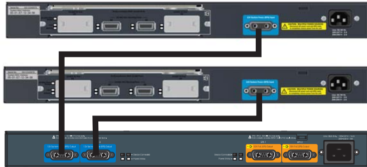
Figure 2-2. Connecting RPS to 2, 24 port switches.
