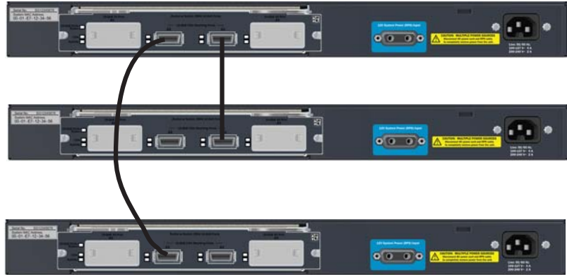
Figure 2-8. Stack of three switches using CX4
