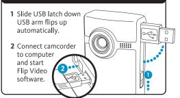
Note: Flip Video program runs directly from the camcorder. Camcorder must be connected while using the software. Battery power is not used while camcorder is connected.
