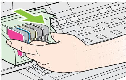
5. Make sure the latch handle is raised, and then reinsert the printhead.
